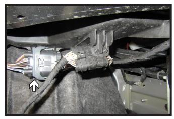
5. Pull the top corners of the fascia out releasing the clips behind, continue working inward towards the grill releasing the clips under the headlights. Pull the fascia forwards, unplug the electrical on the passenger side of the vehicle. Remove fascia and set aside to be reinstalled later.
