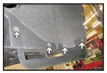
7. Using an 8MM socket, remove the four (4) bolts in front of the tire. Do this on both sides of the vehicle.
