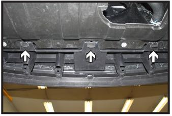
5. On the underside of the fascia, turn the three (3) locking knobs 90° to release.
