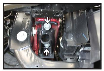
Models equipped with tow hooks: Using a 16MM socket, remove the two (2) bolts from the tow hook bracket. Remove the tow hook bracket from the vehicle. Do this on both sides of the vehicle.
