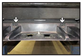
10. Remove the two (2) push pins from the top of the plastic shielding.
