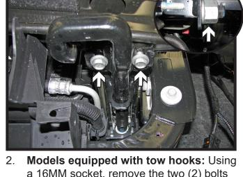
2. **Models equipped with tow hooks:** Using a 16MM socket, remove the two (2) bolts from the front side. Then using a 30MM socket or wrench, remove the nut from the backside of the tow hook. Remove the tow hook from the vehicle. Do this on both sides of the vehicle.
