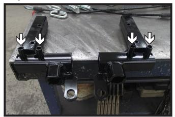
1. Prior to installing the baseplate on the vehicle, install the appropriate spacer tubes into the slots of the baseplate. The tubes will vary depending on whether the vehicle is equipped with tow hooks or not. Reference page 3.
