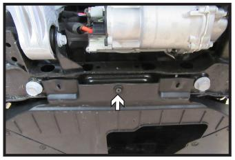
Remove the one (1) push pin from the back center of the plastic belly pan.
