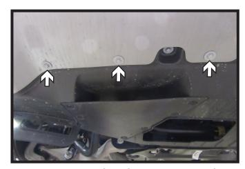
3. Using a 10MM socket, remove the ten (10) bolts on the underside of the fascia. There are five (5) on each side of the vehicle.
