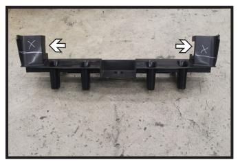
7a. **2014-2020 Models:** Trim the plastic support on the backside of the fascia as shown for baseplate clearance.
