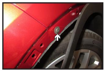
5. Using a T15 Torx, remove the one (1) bolt from the fascia joint under the fender trim. Do this on both sides of the vehicle.
