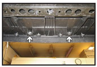
7. Using a 7MM socket, remove the two (2) bolts from center on the underside of the vehicle.
