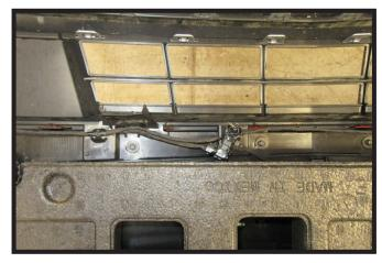
14. Remove the temperature sensor from the bracket on the back side of the fascia. Using a reciprocating saw, cut the bracket as shown. Relocate temperature sensor, connecting it to upper wire loom using the provided zip tie.
