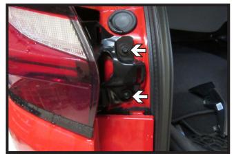
Using a 7MM socket, remove the two (2) bolts attaching the tail light to the frame. To remove, push tail light side ways slightly to unsnap and then pull straight back. Do this on both sides of the vehicle.
