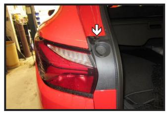
1. Next to the tail light, pull on the black piece from the top to remove. Do this on both sides of the vehicle.
