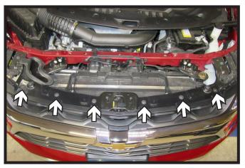
2. Using a T15 Torx, remove the six (6) bolts from the top of the fascia.
