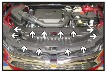
1. Remove the twelve (12) push pins from the fascia cover. Remove fascia cover and set aside to be reinstalled later.
