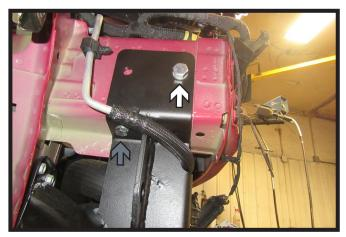
16. Install a 1/2" bolt (white) with lock washer and whiz nut into the front side hole. Then install a 3/8" bolt (gray) with lock washer and whiz nut in back bottom hole. Tighten.
