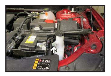
11. Using a 10MM socket, remove the three (3) bolts (white) and one (1) nut (gray) from the windshield washer fluid reservoir on the driver side of the vehicle. Disconnect and unplug all lines. Remove reservoir and set aside to be reinstalled later.
