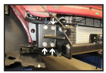
19. Hold the driver side plate and cross bar in place. Where the cross bar attaches to the passenger side plate, start the four (4) 1/2" bolts and hardware. Hand tighten. Use a vise grip to hold the driver side plate in place.
