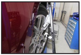
4. Pull back the wheel well trim past the fascia joint. Prop trim away from the vehicle using a soft cloth. Unplug the electrical connection. Do this on both sides of the vehicle.
