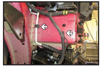
13. Unclip the two lines from the frame on the driver side of the vehicle.
