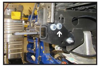
20. Install 1/2" bolt with lock washer with flat washer and whiz nut. Tighten 1/2" then tighten rear 5/8" bolt. Do this on both sides of the vehicle.
