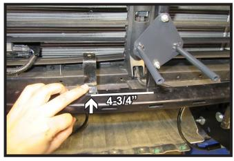
23. **Optional**: Measure 4-3/4" from the center and mark. Using a 1/4" drill bit, drill a hole in the cross member. Install breakaway bracket using the provided 1/4" bolt with hardware.
