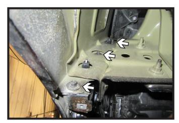
4. Pull back the wheel well liner. Using a 7MM socket, remove the three (3) bolts from the fascia joint. Do this on both sides of the vehicle.
