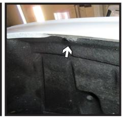
3b. **GMC Models**: Using a T15 Torx, remove the seven (7) bolts from the wheel well edge. Do this on both sides of the vehicle.
