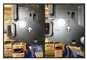
19. Using a 1/2" drill bit, drill out the top back hole in the frame using the baseplate as a template. Do this on both sides of the vehicle.
