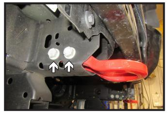
Using am 18MM socket and wrench, remove the two (2) bolts from the tow hook. Set tow hook aside, it will not be reinstalled. Do this on both sides of the vehicle.
