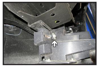
5a. **Chevy Models**: Pull back wheel well liner. Using a 10MM socket, remove the one (1) bolt behind the fascia in front of the tire. Do this on both sides of the vehicle.
