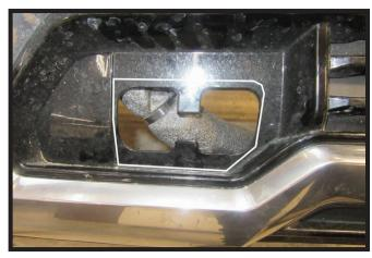
26b. **GMC Models**: Using a reciprocating saw, trim the tow hook opening on the fascia as shown. Do this on both sides of the vehicle.
