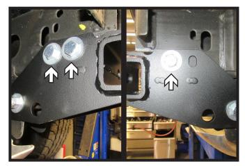
18. Install three (3) 1/2" bolts with flat washers and whiz nuts. Tighten inside bolts then outside bolts. Do this on both sides of the vehicle.
