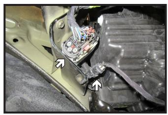
8. As the fascia is removed, unplug the two (2) electrical connections on the passenger side of the vehicle. Remove fascia and set aside to be reinstalled later.
