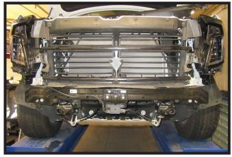
25. Reinstall bumper. Reattach the ACC bracket and wire loom(s) to the bumper.
