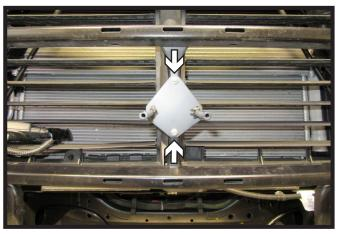
22. Mount the electrical bracket to the top center support brace using the two (2) provide 1/4" bolts with hardware.
