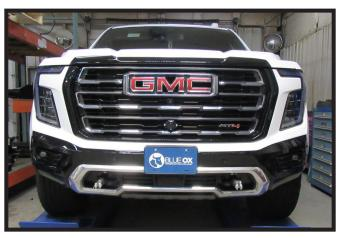
27. Reinstall bottom bolts and tighten upper nuts on top shutter housing. Reinstall the fascia, fascia cover, and hood latch handle. Reconnect all electrical connections.
