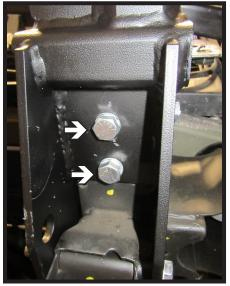
16. Insert two (2) 1/2" x 1-1/2" bolts with lock washers and whiz nuts into bottom holes and tighten. Do this on both sides of the vehicle.
