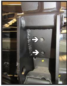
15. Ensure baseplate is flat flush with the bottom of the frame. Using a 1/2" drill bit, drill out the two (2) holes in the bottom of the frame using the baseplate at a template. Do this on both sides of the vehicle.
