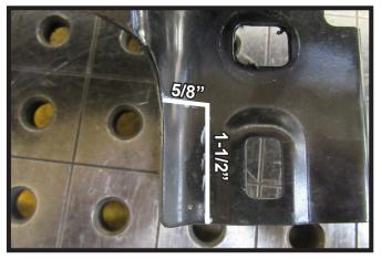
24. On the passenger side of the bumper a measure 5/8" x 1-1/2" area as shown.Using a reciprocating saw trim the indicated area.
