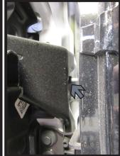
10. Using a 10MM socket, remove the bottom bolt (white) and loosen the top nut (gray) from the upper shutter housing. Do this on both sides of the vehicle.
