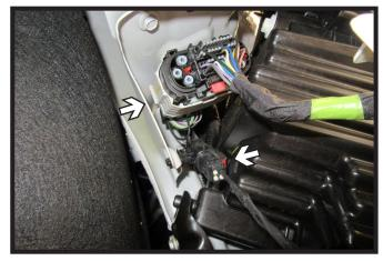
7a. **Gas Models**: As the fascia is removed, unplug the two (2) electrical connections on the passenger side. Remove fascia and set aside to be reinstalled later.
