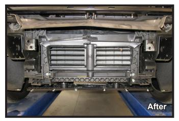
13. **Diesel Models**: Using a reciprocating saw, trim the rubber shroud around the lower shutters as shown to allow for baseplate clearance.
