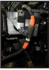
7b. **Diesel Models**: As the fascia is removed, unplug the two (2) electrical connections on the passenger side (white) and one (1) electrical connection on the driver side (gray). Remove fascia and set aside to be reinstalled later.
