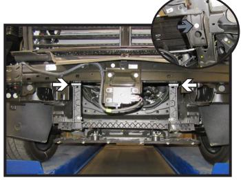
8. **Gas Models**: Using a reciprocating saw, cut the top of the plastic piece on each side as indicated. Then using a 10MM socket, remove the two (2) bolts, one (1) on each side, from the bottom of the plastic piece (inset). Remove plastic piece, it will not be reinstalled.
