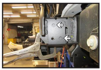
16. Using a 1/2" drill bit, drill out the driver side holes in the frame using the baseplate as a template. Then ream out the existing holes on both side of the vehicle using a 1/2" drill bit.
