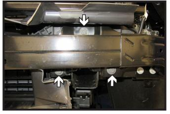
12. Using a 15MM socket, remove the six (6) bolts, three (3) on each side from the bumper. Unclip wire loom on driver side of the bumper if present. Remove bumper and set aside to be reinstalled later.
