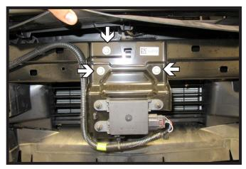
11. Using a 10MM socket, remove the three (3) bolts attaching the adaptive cruise control (ACC) bracket to the bumper. Unclip wire loom from the bumper. Set ACC sensor with bracket out of the way for baseplate installation.
