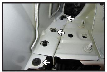
4. Pull back the wheel well liner. Using a 7MM socket, remove the three (3) bolts from the fascia joint. Do this on both sides of the vehicle
