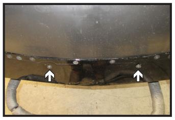
17. Using a T15 Torx, remove the two (2) bolts from the underside of the fascia.
