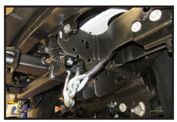
14. Attach the permanent baseplate safety cables to the provided convenience link on the baseplate. The photo above shows the recommended installation of the cables to frame of vehicle. Additional options may interfere with suggested mounting; in this case, secure the cables to a solid piece of the frame as described in the General Information sheet. Be sure the safety cables do not rub against any hoses or moving parts. Do this on **BOTH** sides of the vehicle.
