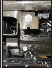
10. Measure 3/4" from the bottom of the bracket and mark a straight line. Using a reciprocating saw, trim off end of bracket to allow for baseplate clearance. Do this on both sides of the vehicle.
