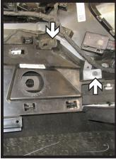
16. Using a 7MM socket, remove the four (4) bolts, two (2) on each side, from the cover on the back of the fascia.
