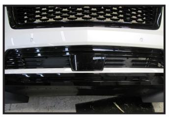
21. Hold the fascia as close to the original position and mark for tabs, convenience links and electrical bracket. Using a reciprocation saw trim marked area as shown. Reinstall the secondary cover on the back of the fascia. Mark using the fascia as a template and trim using a reciprocating saw.
