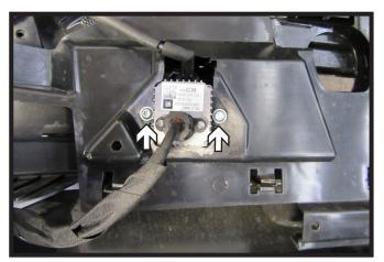
15. Using a T25 Torx, remove the two (2) bolts attaching the sensor to the back of the fascia on the driver side.
