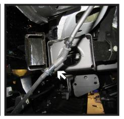
7. As the fascia is removed, uplug the two (2) electrical connections on the passenger side and one (1) on the driver side. Then disconnect the hose on the driver side of the vehicle. Remove fascia and set aside to be reinstalled later.
