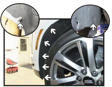
3. Using a T15 Torx, remove the seven (7) bolts from the wheel well. Do this on both sides of the vehicle.
