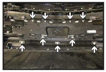
20. Remove the nine (9) clips, five (5) on the bottom and four (4) on the top, from the secondary cover on the back of the fascia. Remove secondary cover and set aside to be reinstalled later.
