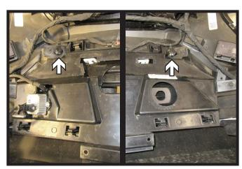
19. Unclip the wire loom on each side from the cover. Remove cover from the back of the fascia and set aside to be reinstalled later.
