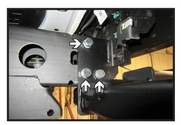
11a. Slide baseplate onto the vehicle and insert three (3) 1/2" bolts with lock washers and whiz nuts into side holes on the driver side of the vehicle. Hand tighten.
