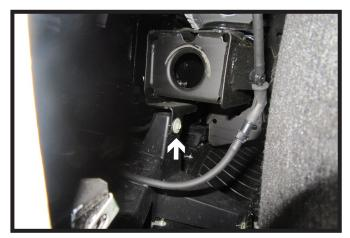
5. Pull back the wheel well liner. Using a 10MM socket, remove the one (1) bolt behind the fascia in front of the tire. Do this on both sides of the vehicle.
