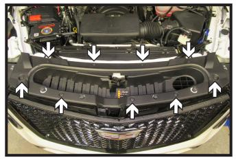
Remove the nine (9) push pins from the fascia cover. Remove fascia cover, and set aside to be reinstalled later.
