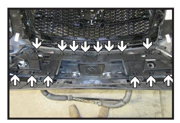
18. Unclip the fourteen clips, six (6) on the bottom and eight (8) on the top, from the cover on the back of the fascia.
