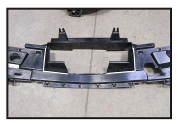
22. Using a reciprocating saw trim the indicated area on the plastic cover and reinstall on the back of the fascia. Mark cover using the fascia as a template and trim using a reciprocating saw.
