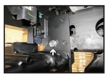
11b. Start one (1) 1/2" bolt with lock washer and whiz nut in the bottom front hole on the passenger side of the vehicle. Hand tighten.
