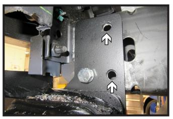
12. Using a 1/2" drill bit, drill the remaining two (2) side holes on the passenger side of the vehicle using the baseplate as a template. Insert two (2) 1/2" bolts with lock washers and whiz nuts. Tighten all side bolts at this time.
