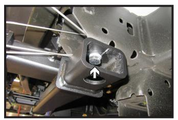
13. Using a 1/2" drill bit, drill the one (1) hole on the bottom of the baseplate using the baseplate as a template. Insert one (1) 1/2" bolt with lock washer and whiz nut. Do this on both sides of the vehicle. Tighten.
