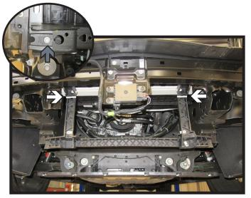
9. Using a reciprocating saw, cut the top of the plastic piece on each side as indicated. Then using a 10MM socket, remove the two (2) bolts, one (1) from each side, from the bottom of the plastic piece (inset). Remove plastic piece, it will not be reinstalled.
