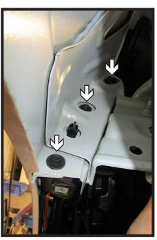
4. Pull back the wheel well liner. Using a 7MM socket, remove the three (3) bolts from the fascia joint. Do this on both sides of the vehicle.
