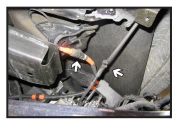
8c. **Diesel Models**: Disconnect the hose and diesel line on the driver side of the vehicle behind the facia. Remove the fascia and set aside to be reinstalled later.
