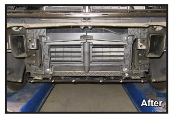
13. **Vehicles with Lower Shutters**: Using a utility knife, remove the shroud around the lower shutters as shown.
