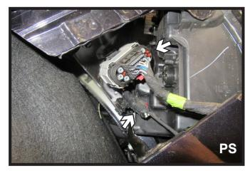
8b. **Diesel Models**: Gently pry the fascia loose from the front end of the vehicle. Unplug the one (1) electrical connections on the driver side and the two (2) electrical connections on the passenger side behind the facia.
