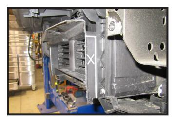
14. Vehicles with Lower Shutters: Using a reciprocating saw, trim each end of the shutter housing as indicated. Do this on both sides of the vehicle.
