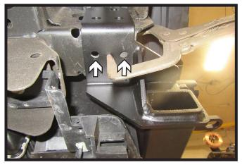
16. Using a 1/2" drill bit, drill out the bottom two (2) holes in the vehicle using the baseplate as a template. Install two (2) 1/2" bolts with lock washers and whiz nuts into the bottom holes, tighten. Do this on both sides of the vehicle.
