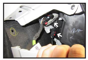
8a. **Gas Models**: Gently pry the fascia loose from the front end of the vehicle. Unplug the two (2) electrical connections on the passenger side behind the facia. Remove the fascia and set aside to be reinstalled later.
