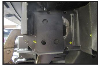
17. Using a 1/2" drill bit, drill out the side holes on the baseplate using the baseplate as a template. Then ream out existing holes. Do this on both sides of the vehicle.
