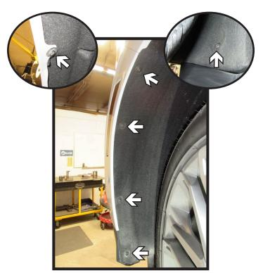
4. Using a T15 Torx, remove the six (6) screws from the wheel well. There are five (5) along the edge and one (1) in front of the tire. Do this on both sides of the vehicle.
