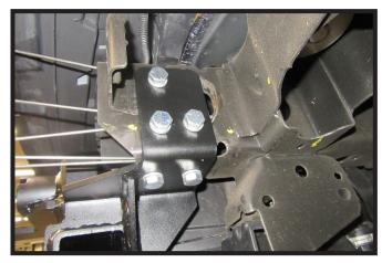
18. Install 1/2" bolts with lock washers and whiz nuts in to side holes and tighten.
