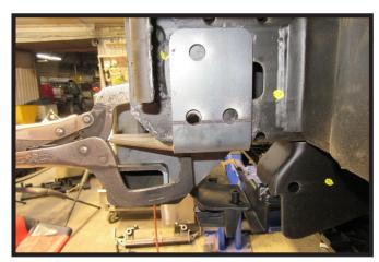
15. Slide the baseplate onto the vehicle lining up the existing hole on each side as close as possible. Hold in place using large vice grips.
