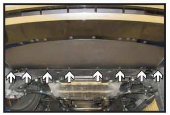
Using a 7MM socket, remove the eight (8) bolts from the underside of the fascia.
