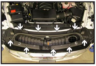
Remove the nine (9) push pins from the top of the fascia. Remove fascia cover and set aside to be reinstalled later.
