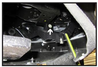
7. Pull back the bottom of the wheel well liner in front of the tire. Using a 10MM socket, remove the one (1) bolt. Do this on both sides of the vehicle.
