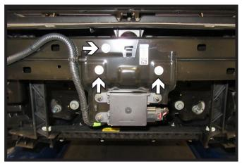
10. Using a 10MM socket, remove the three (3) bolts from the Adaptive Cruise Control (ACC) mounting bracket. Unclip wire loom from the bumper on the passenger side. Set sensor and wire loom out of the way on top of the engine compartment.
