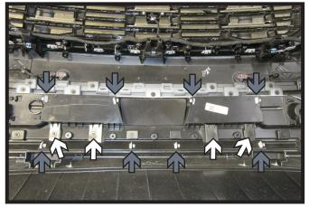
Using a 7MM socket remove the four (4) bolts (white) below the tow hook covers.
