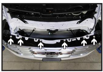
3. Using a 10MM socket, remove the six (6) bolts from the top of the fascia.
