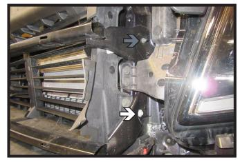
11. Using a 10MM socket, remove the bottom bolt (white) and loosen the top nut (gray) from the upper shutter housing. Do this on both sides of the vehicle.
