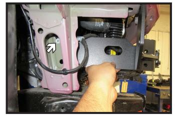
17. Hold the support plate in place as shown on passenger side of the vehicle so the front holes and back bottom hole line up with the existing holes on the vehicle. Mark frame using the baseplate as a template for top back hole.
