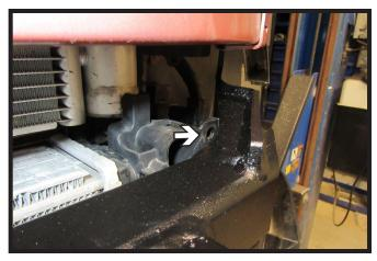
16. **Optional**: If needed trim the indicated corner plastic piece to allow for baseplate clearance.
