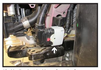
19. Unclip electrical loom from the frame on driver side of the vehicle to allow for installation of support plate.
