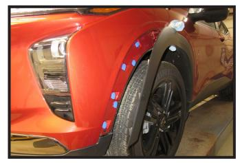
Pull back the wheel well trim, releasing the nine (9) push pins, past the fascia joint.
