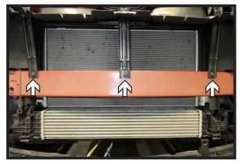
11. **Optional**: Using a 10MM socket, remove the three (3) bolts from the bumper support brackets. Remove bumper and set aside to be reinstalled later.
