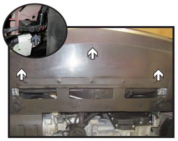
7. Using a T15 Torx, remove the three (3) bolts from the bottom of the fascia. Then disconnect the electrical on the driver side of the vehicle (inset). Remove fascia and set aside to be reinstalled later.
