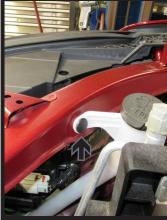
9. Using a 10MM socket, remove the two (2) nuts (white), one (1) bolt (gray), and one (1) push pin (black) from the windshield washer fluid reservoir on the passenger side of the vehicle. Disconnect and plug all lines. Disconnect the two (2) electrical connections. Remove reservoir and set aside to be reinstalled later.
