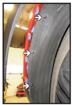
4. Using a T15 Torx, remove the three (3) bolts from the wheel well edge. Do this on both sides of the vehicle.
