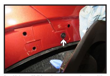
Using a 7MM socket, remove the one (1) bolt from the fascia joint. Do this on both sides of the vehicle.
