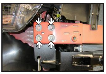
15. Start the remaining three (3) existing bolts. Do this on both sides of the vehicle. Ensure the baseplate is level and tighten all eight (8) bolts, four (4) on each side.
