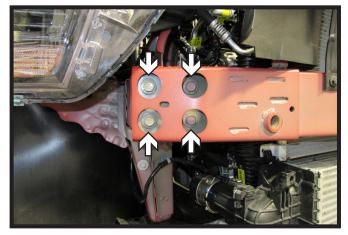
10. Using a 15MM socket, remove the four(4) bolts from the bumper. Do this on both sides of the vehicle. Let hang from support brackets.
