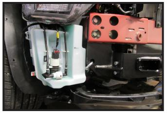
Reinstall windshield washer fluid reservoir, reconnecting all lines and electrical connections.
