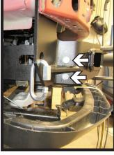
20. Slide support plate onto the vehicle toward the inside of the frame and baseplate. Start two (2) 3/8" bolts (white) with nylon lock nuts into front holes. Then start two (2) 1/2" bolts (gray) with lock washers, flat washers, and wire nuts in back holes. Tighten back 1/2" bolts then front 3/8" bolts. Do this on both sides of the vehicle.
