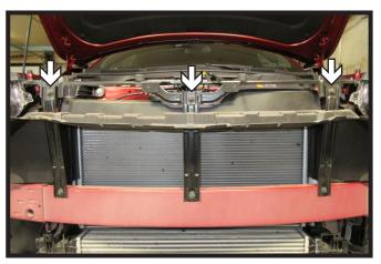
13. **Optional**: Reattach bumper to support brackets, leave loose. Then using a 10MM socket, loosen the top three (3) support bracket bolts.
