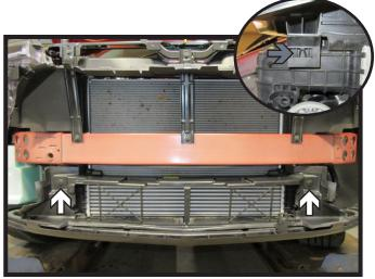
8. Remove the two (2) push pins, one (1) on each side from the plastic shroud. Then release the clip from the bottom of shroud, there is one (1) on each side (inset). Remove shroud, it will not be reinstalled.
