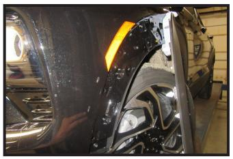
Pull back the wheel well trim, releasing the ten (10) push pins, past the fascia joint.
