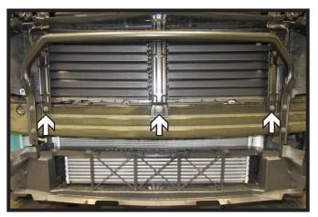
Using a 10MM socket, remove the three
