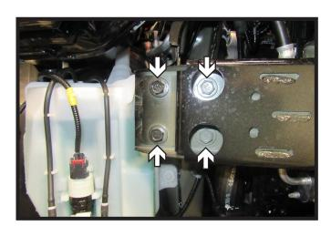
Using a 15MM socket, remove the four (4) bolts from the bumper. Do this on both sides of the bumper. Remove bumper and set aside to be reinstalled later.
