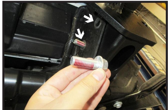
15. Slide baseplate onto vehicle so that the convenience link is to the outside of the vehicle (left). To ensure holes line up, start the four (4) 1 1/2" x 1-1/2" whiz flange bolts (right). Do this on both sides of the vehicle.
