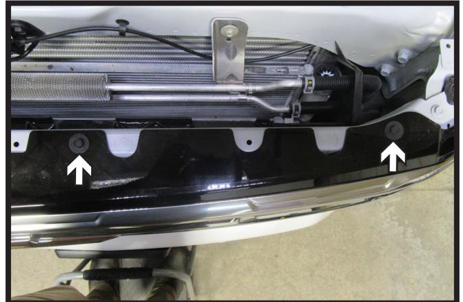
3. Using a 10MM socket, remove the four (4) bolts from the top of the fascia.
