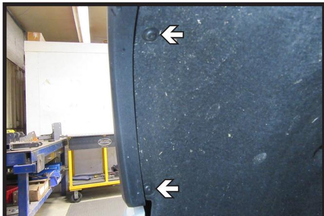
4. Using a T15 Torx, remove the two (2) bolts from along the edge of the wheel well. Do this on both sides of the vehicle.
