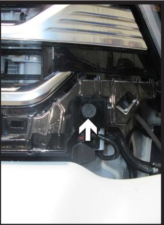
8. Using a 10MM socket, remove the one (1) bolt from the bottom corner of the grille on each side of the vehicle.
