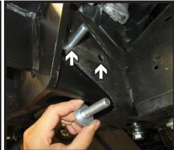
13. Slide baseplate onto vehicle so that the convenience link is to the outside of the vehicle (left). To ensure holes line up, start the two (2) 1/2" x 1-1/2" whiz flange bolts towards the inside (center) and the two (2) 1/2" x 2" with flat washer towards the outside of the vehicle (right). Do this on both sides of the vehicle.
