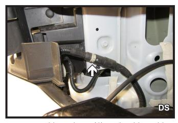
12. Unplug the one (1) electrical connection on the passenger side and one (1) on the driver side. Remove bumper and set aside to be reinstalled later.
