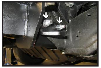
15. Slide the baseplate safety cable bracket onto the two (2) 1/2" outer bolts and place a nylon lock nut on each bolt to secure. Fully tighten. Do this on both sides of the vehicle.
