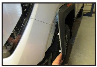
5. Pull back the wheel well trim past the fascia joint. Prop trim away from the vehicle using a soft cloth. Do this on both sides of the vehicle.
