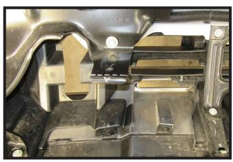
20. Using a reciprocating saw, trim the metal bracket on the back of the bumper as shown. Do this on both sides of the vehicle.
