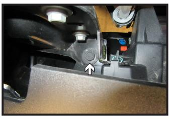
11. On the top side of the bumper, use an 18MM socket and socket extension to remove the two (2) bolts from behind the bumper. Do this on both sides of the vehicle.
