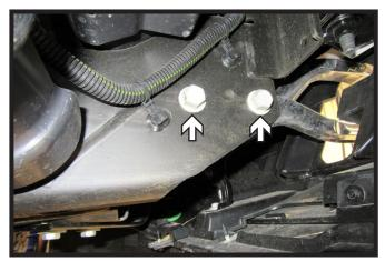
9. Using an 18MM socket and a wrench, remove the two (2) bolts from the tow hook. Do this on both sides of the vehicle. Remove tow hooks, they will not be reinstalled.
