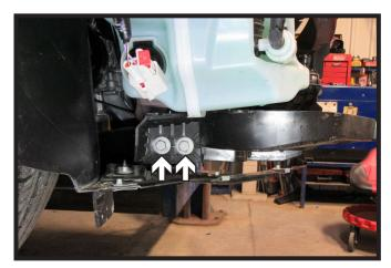
11. Using a 13MM socket, remove the two (2) bolts from plastic piece below the windshield washer reservoir. Do this on both sides of the vehicle. Remove piece and set aside to be reinstalled later.
