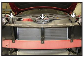
15. Reattach bumper to support brackets, leave loose. Then using a 10MM socket, loosen the top three (3) support bracket bolts
