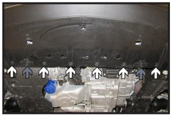
6. Using a 7MM socket, remove the six (6) bolts (white) from the bottom of the fascia. Then remove the two (2) push pins (gray).
