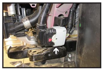
Unclip electrical loom from frame on driver side of the vehicle to allow for installation of support plate.
