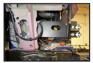
21. Slide support plate onto the vehicle toward the inside of the frame and baseplate. Start two (2) 3/8" bolts (white) with nylon lock nuts into front holes. Then start two (2) 1/2" bolts (gray) with lock washers, flat washers, and wire nuts in back holes. Tighten back 1/2" bolts then front 3/8" bolts. Do this on both sides of the vehicle.
