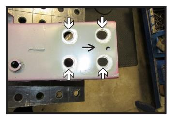
14. Slightly slot the four (4) holes in the bumper towards the outside. Do this on both sides of the bumper.
