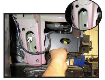
18. Hold the support plate in place as shown on passenger side of the vehicle so the front holes and back bottom hole line up with the existing holes on the vehicle. Mark frame using the baseplate as a template for top back hole.
