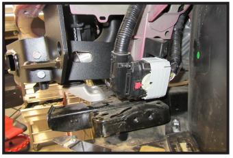
22. Reattach electrical loom to frame on the driver side of the vehicle.
