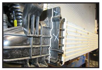
Using a reciprocating saw, trim the plastic as shown for baseplate clearance. Do this on both sides of the vehicle.
