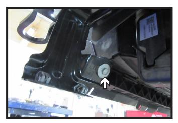
17. Using a 10MM socket, remove the one (1) bolt from the back of the lower shutters on the driver side of the vehicle.
