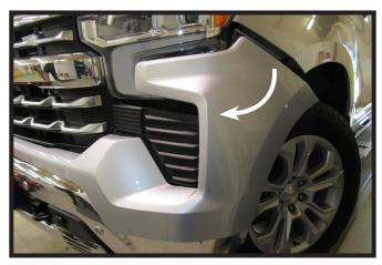
Starting on one side of the vehicle, lift and pull the center fascia piece way from the vehicle. Then unsnap piece across the front of the vehicle and finally lifting and pulling piece away from other side. Set center fascia piece aside to be reinstalled later.
