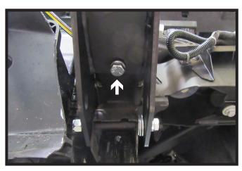
22. Install a 1/2" bolt with lock washer on bottom and a flat washer with whiz nut on top into bottom hole of the baseplate. Do this on both sides of the vehicle. Remove side bolts, apply Loctite Red and reinstall. Do this on both sides of the vehicle.
