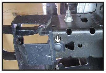
16. Remove the one (1) push pin from the bottom of the tow hook cover. Remove cover from the tow hook, it will not be reinstalled. Do this on both sides of the vehicle.
