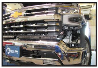
30. Reinstall upper grille piece and reconnect remaining electrical connections.
