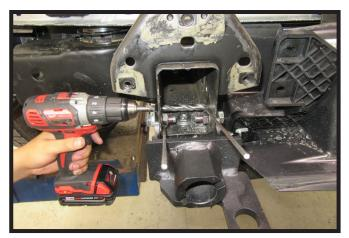
24. Using a 1/2" drill bit, drill the top rear inside hole on the passenger side of the vehicle, using the baseplate as a template. Drill straight through the tow hook housing from the rear outside hole to drill rear inside hole.
