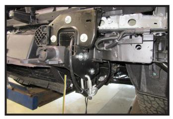
26. Attach the permanent baseplate safety cables to the provided convenience link on the baseplate. The photo above shows the recommended installation of the cables to frame of vehicle. Additional options may interfere with suggested mounting; in this case, secure the cables to a solid piece of the frame as described in the General Information sheet. Be sure the safety cables do not rub against any hoses or moving parts. Do this on **BOTH** sides of the vehicle.
