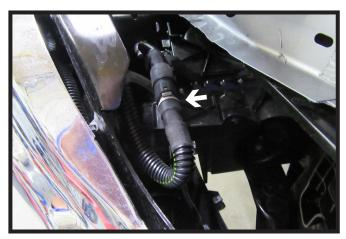
11. Unplug the electrical on the driver side of the vehicle.
