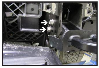
Using an 18MM socket, remove the two
