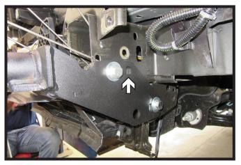
23. Using a 1/2" drill bit, drill the top rear outside hole on the driver side of the vehicle, using the baseplate as a template.
