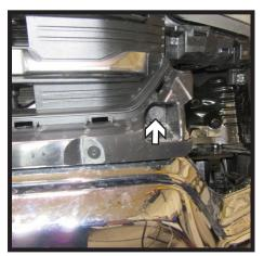
7. Using a 10MM socket, remove the three (3) bolts from the bottom edge of the grille piece. There is one (1) bolt on each side and one (1) in the center.
