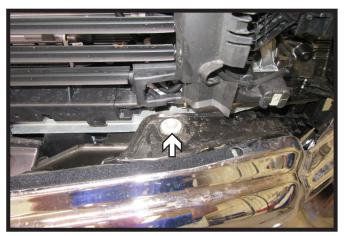
10. Using an 18MM socket, remove the two(2) bolts from the top edge of the bumper.There is one (1) on each side.
