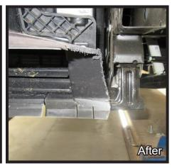
19. Using a reciprocating saw, trim the shutter housing as shown. Do this on both sides of the vehicle.
