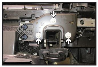
15. Using a 15MM socket, remove the three (3) bolts (white) from the front of the tow hook housing. Then using a 7MM socket, remove the two (2) bolts (gray). Remove front piece and set aside to be reinstalled later. Do this on both sides of the vehicle.
