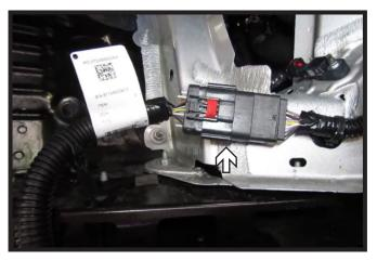
12. Unplug the electrical on the passenger side of the vehicle.
