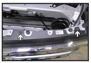
3. Using a 7MM socket, remove the four (4) bolts, two (2) on each side from the top of the fascia.
