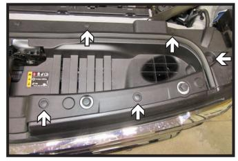
2. Remove the ten (10) push pins from along the top of the fascia. Remove fascia cover and set aside to be reinstalled later.
