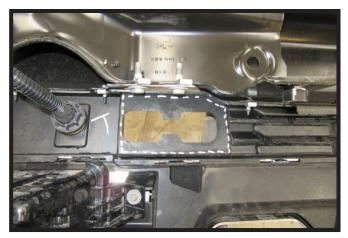
28. Using a reciprocating saw, trim the indicated area around tow hook opening on the back of the bumper to allow clearance for baseplate. Do this on both sides of the vehicle. Reinstall bumper and reconnect electrical.
