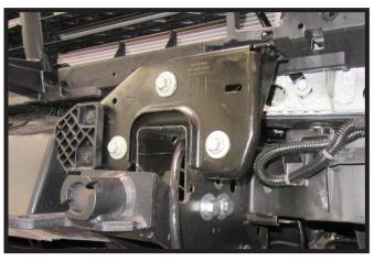
27. Reinstall the tow hook housing front plate. Then reinstall lower shutter bolt on driver side of the vehicle.
