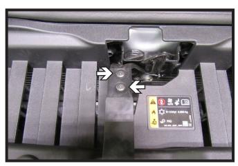
Using a T15 Torx, remove the two (2) bolts from the handle on the top edge of the fascia. Remove and set aside to be reinstalled later.
