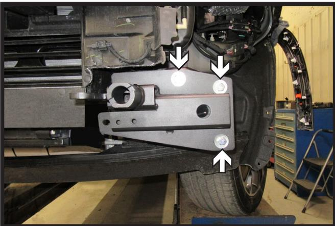
10. Hold baseplate in place and start the three (3) 1/2" x 1-1/2" bolts with flat washers and nylon lock nuts. Snug up the baseplate into place but leave loose. Do this on both sides of the vehicle.
