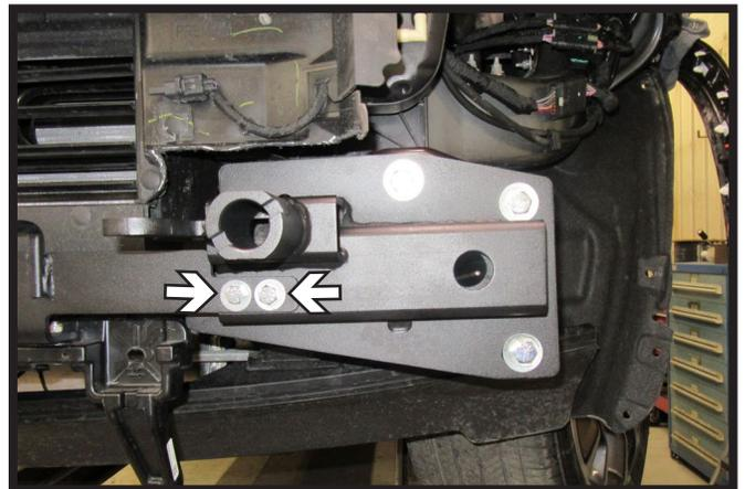
11. Attach cross member to baseplates, start the two (2) 3/8" x 1" bolts with flat washers and nylon lock washers. Do this on both sides of the vehicle. Ensure baseplate is level and tighten baseplate on each side then cross member.
