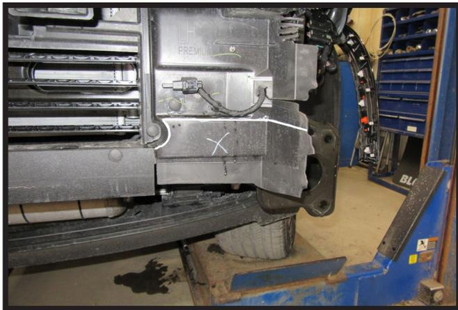
6. Using a utility knife, trim plastic shroud as shown on both sides of the vehicle and remove piece.
