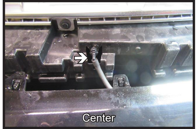
5. Remove fascia and set aside to be reinstalled later. Unplug the electrical on both sides of the vehicle and hose in the center as the fascia is removed.
