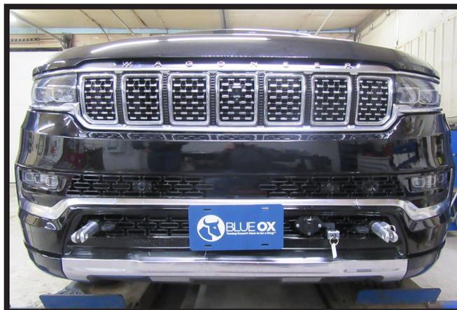
18. Hold the fascia as close to its original position, mark and trim the fascia around the convenience links and attachment tabs. Reinstall the fascia and reconnect all electrical and hose.
