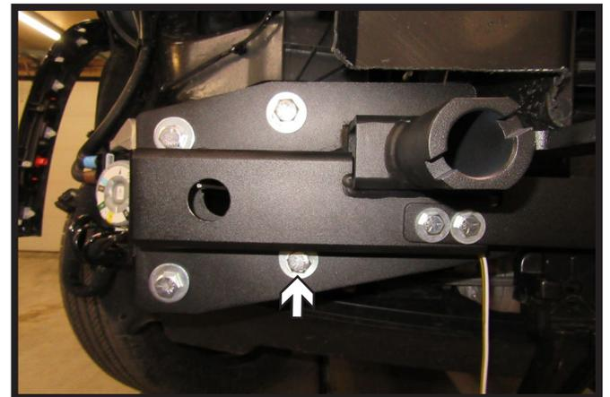
15. Install one (1) 1/2" x 1-1/2" bolt with flat washer and nylon lock nuts into the bottom inside hole on the front of the baseplate. Do this on both sides of the vehicle.
