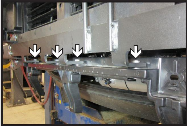
16. Attach plastic piece from bumper to cross member using four (4) 1/4" x 1" bolts with flat washers and lock washers.
