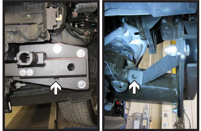
13. Using a 1/2" drill bit, drill the bottom inside hole on the front of the baseplate (left). Then using the support bracket as a template, drill 1/2" hole in frame (right). Do this on both sides of the vehicle.
