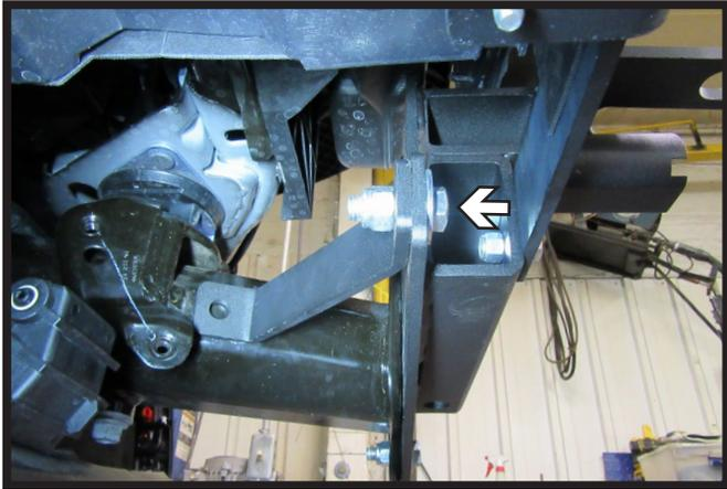
12. Attach support bracket to baseplate using one (1) 1/2" x 1-1/2" bolt with flat washer and nylon lock nut. Do this on both sides of the vehicle.
