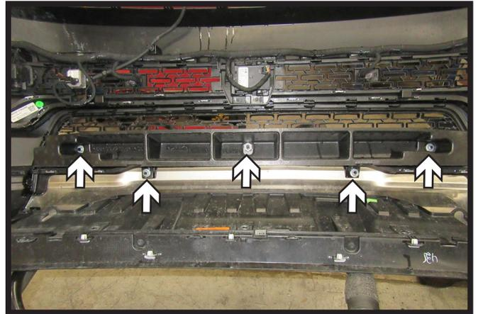
9. Using a 13MM socket, remove the five (5) nuts on the backside of the fascia. Remove foam piece and set aside. It will not be reinstalled.
