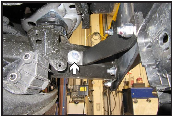
14. Install one (1) 1/2" bolt with lock washer and whiz nut. Do this on both sides of the vehicle.
