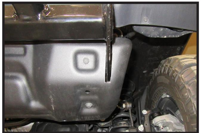
12. Trim belly pan for baseplate clearance in one of two ways listed below then reinstall belly pan. **Note:** For Sport, Sport S, and Overland models the skid plate will need to be reinstalled before the belly pan.
