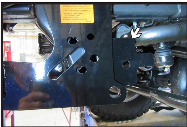
9b. **All Other Models:** Place the spacer plate between the frame and the baseplate. May need to use a pry bar to allow more room for the spacer plate to slide into place. Install the two (2) 3/8" bolts with hardware (white). Then install the one (1) 1/2" bolt with hardware into the bottom back hole. May need to ream out the bottom back hole. Do this on both sides of the vehicle.
