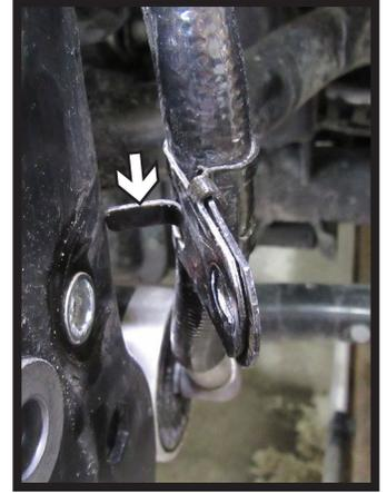
Pull hose clamp away from frame and straighten the rear tab as shown. (Right)
