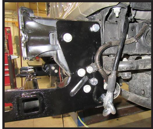
10. **All Models:** Using a 1/2" drill bit, drill the top back hole using the baseplate as a guide. Install the one (1) 1/2" bolt with hardware. Do this on both sides of the vehicle.
