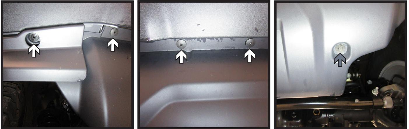
2c. **Sport & Sport S Models:** Remove the eight (8) push pins from the front edge of the belly pan, there are four (4) on each side (white). Then using an 8MM socket, remove the two (2) bolts (gray), one (1) on each side, from the belly pan. Remove belly pan and set aside to be reinstalled later.
