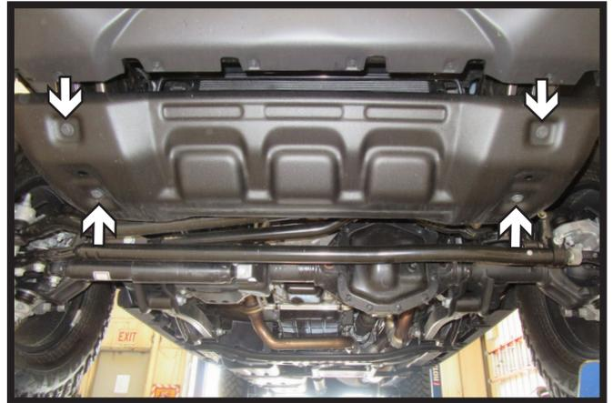
2a. **Rubicon w/Plastic Bumper Models:** Using a 13MM socket, remove the four (4) bolts from the belly pan. Remove belly pan and set aside to be reinstalled later.
