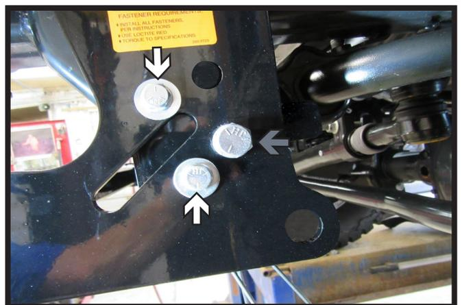
**\*\* Use Loctite® Red on all bolt threads and tighten all bolts to the appropriate torque. \*\***
