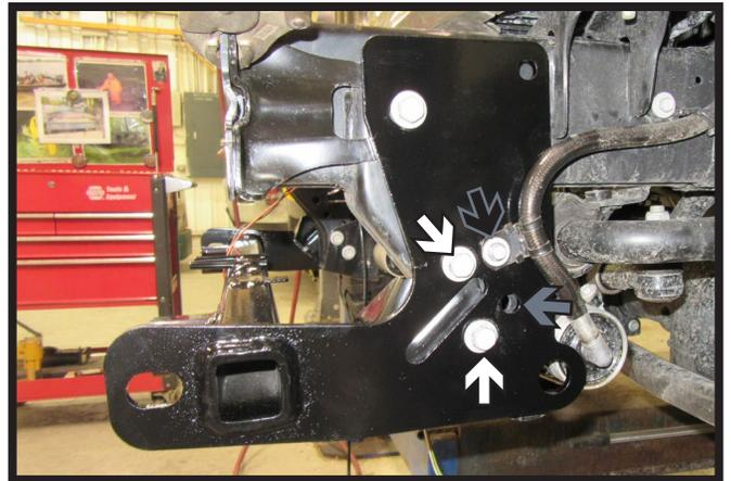
9a. **Rubicon w/Steel Belly Pan Models:** Place the belly pan bracket between the frame and the baseplate. Install the two (2) existing 10MM bolts (white). Then install the one (1) 1/2" bolt with hardware into the bottom back hole (gray). May need to ream out the bottom back hole. **Mojave Models Only:** Install the one (1) existing 6MM bolt (black). Do this on both sides of the vehicle.
