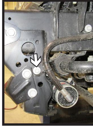
6b. **Mojave Model:** Using a 10MM socket, remove the bolt holding the hose clamp. (Left)
