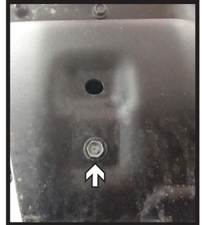
2b. **Rubicon w/Steel Bumper Models:** Using an 13MM socket, remove the seven (7) bolts from the belly pan. There are five (5) bolts along the front edge (left and center) and two (2) in the back (right). Remove belly pan and set aside to be reinstalled later.
