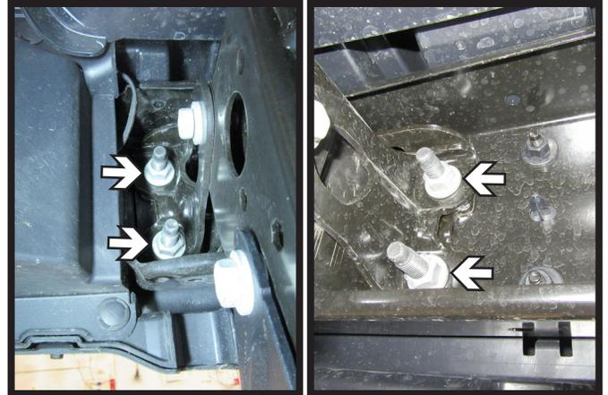
5. Using an 18MM socket, remove the four (4) nuts holding the bumper to the frame. Do this on both sides of the vehicle. Remove the bumper and set aside to be reinstalled later.
