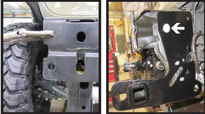
8. Hold frame bracket in place with vice grip (Left). Slide baseplate into position and start the top front 10MM existing bolt with hardware (Right). Ensure that all holes line up and the baseplate is level, then snug down bolt. Do this on both sides of the vehicle.
