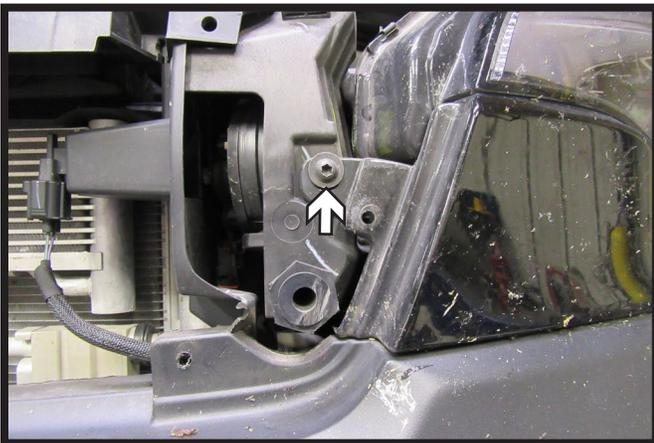
2. Using a T27 Torx, remove the one (1) screw from behind the fascia cover. Do this on both sides of the vehicle.
