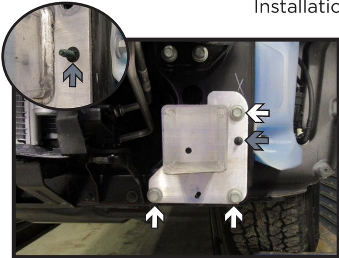
7. Using a 15MM socket, remove the three (3) bolts from the frame extension. Using a 10MM socket, remove the nut (gray) from the frame extension. Do this on both sides of the vehicle. Remove frame extension, it will not be reinstalled.
