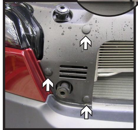
1. Remove the thirteen (13) push pins from the top edge of the fascia cover. There are six (6) on each side and one (1) in the center. Remove fascia cover and set aside to be reinstalled later.
