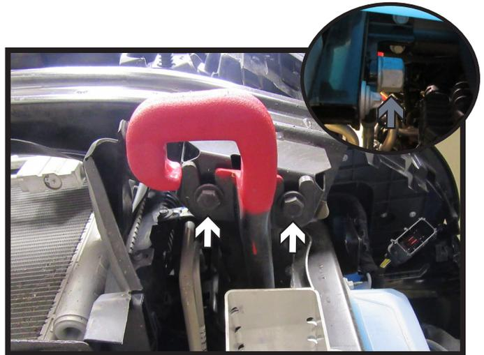
6. Using a 16MM socket, remove the two (2) bolts (white) from the underside of the tow hook. Using a 30MM socket, remove the nut (gray) from the backside of the tow hook (inset). Do this on both sides of the vehicle. Remove tow hooks and set aside, they will not be reinstalled.
