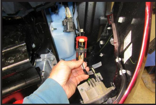
5. Lift the corner of the fascia up towards the fender and out to release. Continue along under the headlights unsnapping the fascia from the vehicle. As the fascia is removed unhook the plug on the driver side by pulling out the yellow piece and up on the red part to unhook. Remove fascia and set aside to be reinstalled later.
