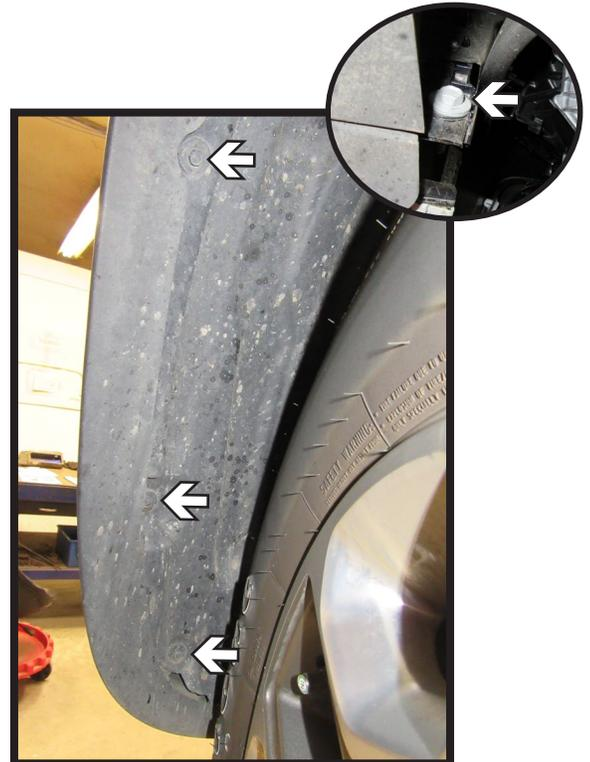
3. Using an 8MM socket, remove the three (3) bolts from the edge of the wheel well. Pull back the wheel well cover, using a 10MM socket, remove the bolt behind the trim (inset). Do this on both sides of the vehicle.
