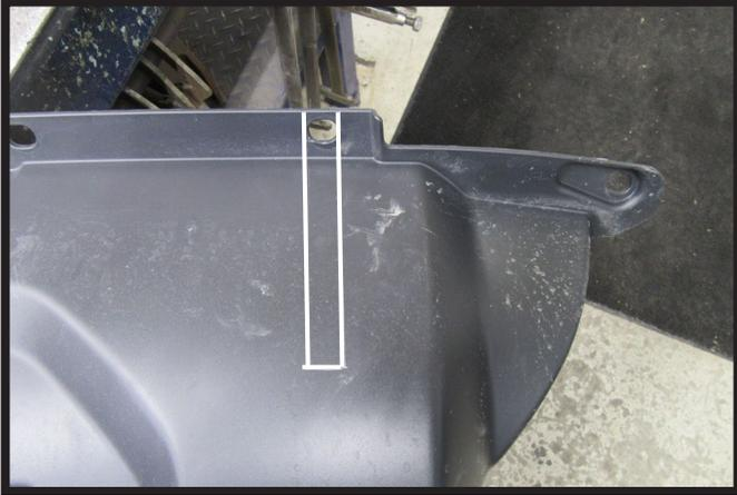
9. Hold the belly pan in place, mark and trim to allow room for the baseplate.
