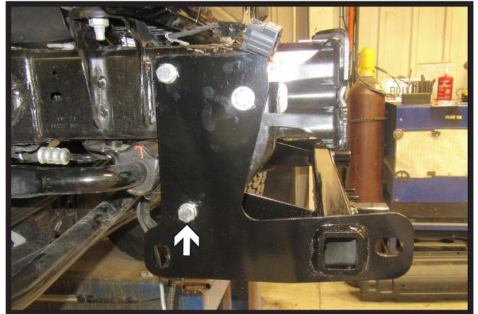
6. Install the 1/2" bolt with lock washer and whiz nut into the bottom hole on the outside of the frame. If the hole does not completely line up ream out hole with drill bit. Do this on both sides of the vehicle.
