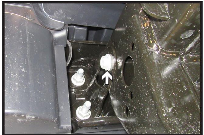
6. Using a 16MM socket, remove the one (1) bolt on the outside of the frame holding the bracket after removing the bumper. Do this on both sides of the vehicle.
