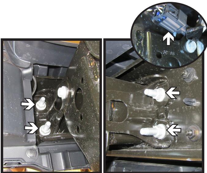
5. Using an 18MM socket, remove the four (4) nuts holding the bumper to the frame. Do this on both sides of the vehicle. On the passenger side of the vehicle unplug the indicated electrical (inset). Remove the bumper and set aside to be reinstalled later.
