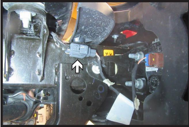
2. On the passenger side of the vehicle unplug the indicated electrical to allow for removal of bumper.
