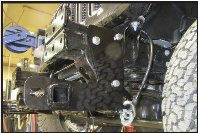
7. Attach the permanent baseplate safety cables to the provided convenience link on the baseplate. The photo above shows the recommended installation of the cables to frame of vehicle. Additional options may interfere with suggested mounting; in this case, secure the cables to a solid piece of the frame as described in the General Information sheet. Be sure the safety cables do not rub against any hoses or moving parts. Do this on **BOTH** sides of the vehicle.
