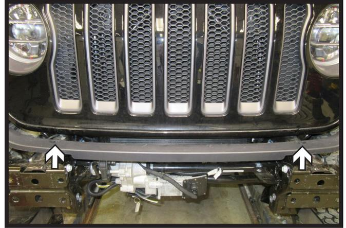
5. Remove the two (2) push pins holding the plastic piece to the frame. Set aside to be reinstalled later.
