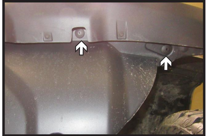
2. Remove the eight (8) push pins from the edge of the belly pan. There are four (4) in the center and two (2) on each side. Remove belly pan and set aside to be reinstalled later.
