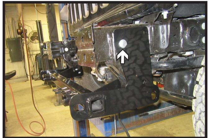
2. Slide the baseplate onto the vehicle. Start the front 10MM bolt with flat washer and lock washer. Snug bolt up tight so remaining holes line up but do not use Loctite® Red at this time. Do this on both sides of the vehicle.
