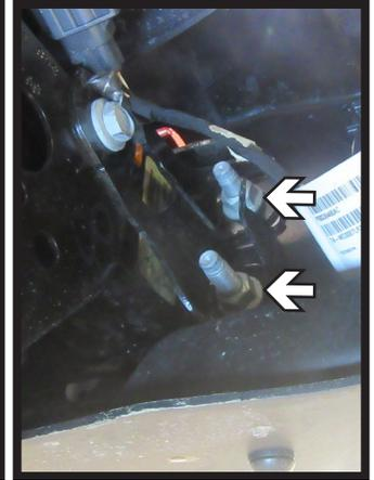
3. Using an 18MM socket, remove the four (4) nuts holding the bumper to the frame. Do this on both sides of the vehicle. Remove the bumper and set aside to be reinstalled later.
