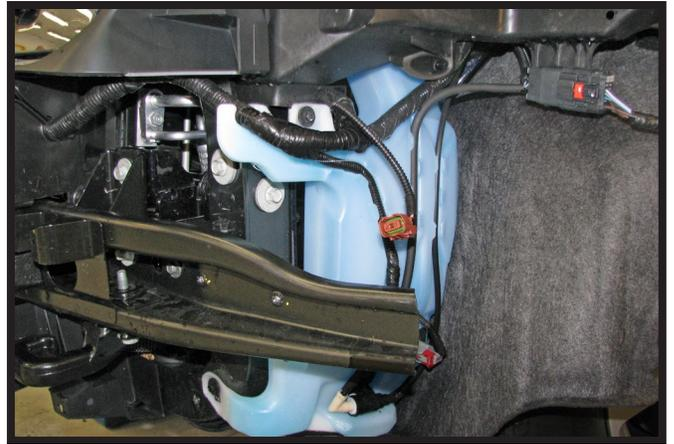
13. Reinstall the washer fluid reservoir and plastic shielding.
