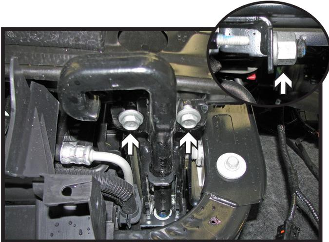
5. **Models equipped with tow hooks:** Using a 16MM socket, remove the two (2) bolts from the front side. Then using a 30MM socket or wrench, remove the nut from the backside of the tow hook. Remove the tow hook from the vehicle. Do this on both sides of the vehicle.
