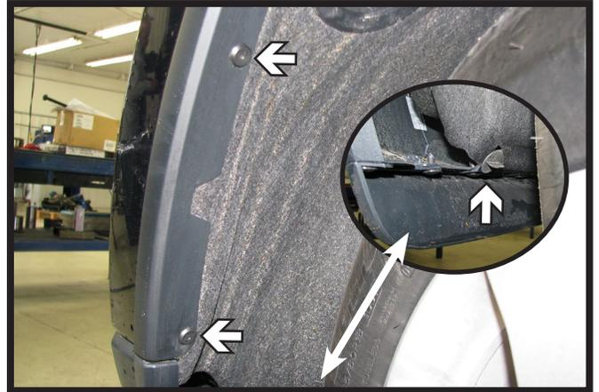
2. Using a utility knife, remove the two (2) plastic rivets from outer edge of the wheel well. Then release the knob at the bottom inner edge of the wheel well, by turning 90°. Do this on both sides of the vehicle.
