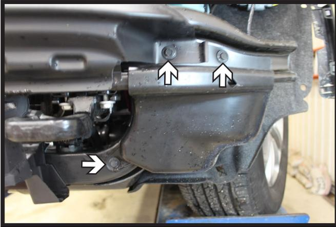
1. If equipped on your model of vehicle, the lower plastic shielding will need to be removed. Using a 10MM socket, remove the three (3) bolts from the shielding. Do this on both sides of the vehicle.
