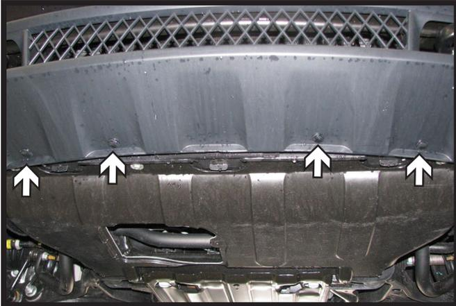
1. On the bottom side of the fascia, remove the four (4) push pins.
