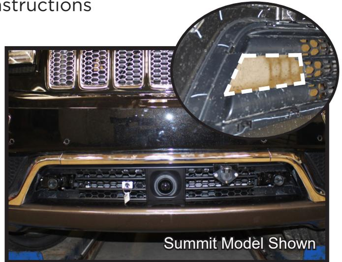
16. Hold the fascia as close to its original position as possible, mark and trim the fascia around the convenience links and attachment tabs. Reinstall the fascia. Using the plastic pop rivet gun, replace the two (2) rivets in the wheel well. Do this on both sides of the vehicle.
