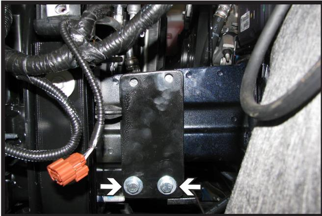
9. With the taper to the front, install the support plate onto the baseplate. Insert the 3/8"-16 x 1-1/2" bolts with 3/8" lock and flat washers into the holes and the 3/8" nut plates on the inside of the baseplate. Flush the top of the plate with the frame and tighten all hardware. Do this on both sides of the vehicle.
