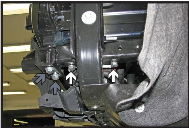
7. **Models equipped with tow hooks:** Slide the baseplate into position on the frame. Install two (2) 10MM-1.5 x 80MM bolts with 10MM lock washers and 3/8" washers into the bottom holes (white). Install a 3/4"Ø x 1-23/32" spacer tube with a 10MM-1.5 x 100MM bolt, 10MM lock and flat washer thru the spacer into the frame into both the front holes (gray). Tighten all hardware. Do this on both sides of the vehicle.
