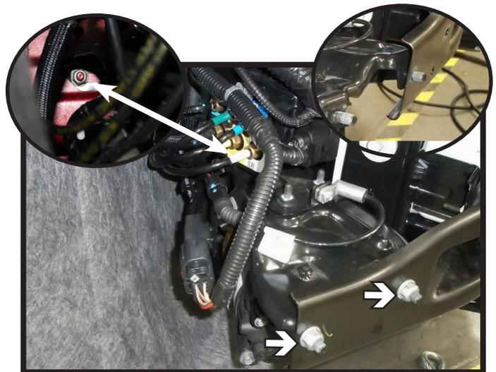
4. On models equipped with a compressor, using a 10MM or 13MM socket, remove the two (2) nuts from the bumper and one (1) nut from the frame behind the compressor (left inset). Move the compressor away from the frame. Put the inner stud into the outer bumper hole and thread on a nut to secure in position (right inset). This will allow room for baseplate installation.
