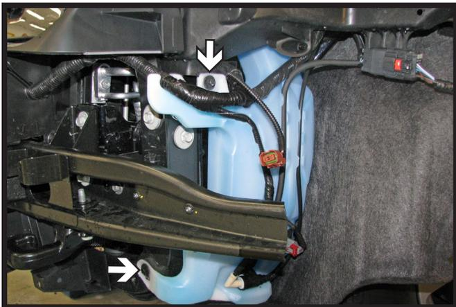
3. Using a 8MM socket, remove the two (2) bolts from the washer fluid reservoir. Disconnect/plug all lines and set reservoir aside.
