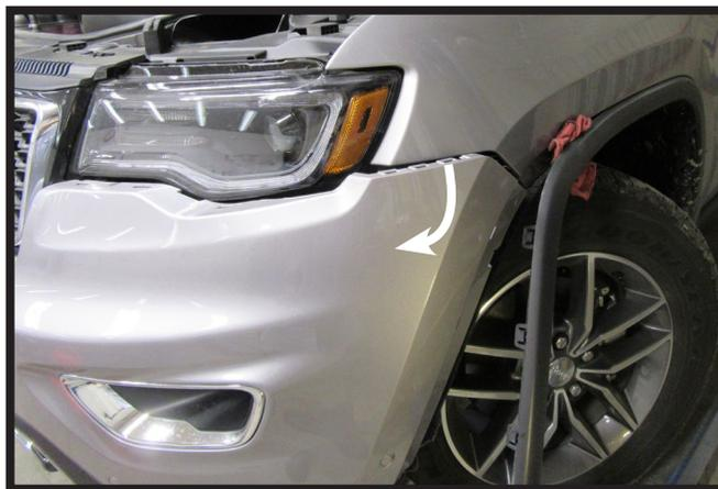
6. Pull the top corners of the fascia out releasing the clips behind. Continue working inward towards the grille releasing the clips under the headlights. Set the fascia aside.
