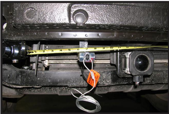
14. **Optional Breakaway:** Measure over approximately 7" from the convenience link or in the desired location, install the bracket to the bumper with a #10-16 x 1" self drilling screw. Attach the breakaway to the bracket with a 1/4"-20 x 3/4" bolt and 1/4"-20 lock nut.
