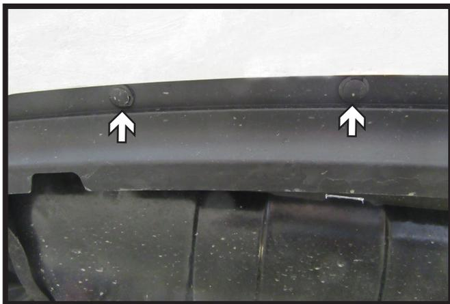
3. Underneath the bumper, remove the two (2) push pins. Do this on both sides of the vehicle.
