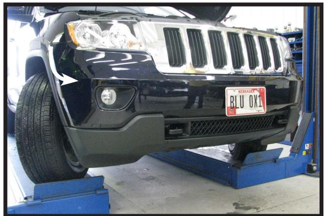
4. Pull the top corners of the fascia out releasing the clips behind. Continue working inward towards the grille releasing the clips under the headlights and grille. Set the fascia aside to be reinstalled later.
