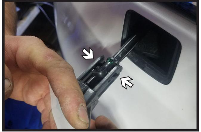
5. For models with headlight sprayers, pull out the square piece to allow the sprayer to be disconnected (left). Press down on the indicated clips on both sides of the bracket to disconnect and remove to be reinstalled later (right). Do this on both sides of the vehicle.
