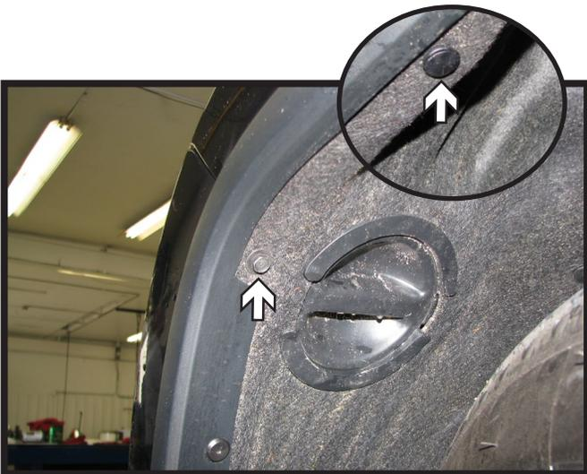
3. Along the upper edge of the wheel well, using a 10MM socket, remove the screw. Then remove the push pin further up (inset). Do this on both sides of the vehicle.
