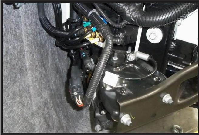
12. Loosely reinstall the compressor, checking for clearance around the baseplate. If needed shim the compressor away from the baseplate with 5/16" washers. This will keep the compressor from vibrating against the baseplate.
