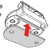
Position the buckle ends (I) with the open side facing the bed cover panel. Use a Phillips screwdriver to install the two buckles into the pre-drilled holes on the front header panel with the provided screws (K) and the nutsert (L) inserted from the backside of the panel. **DO NOT use a screw gun, securely tighten by hand only.**
