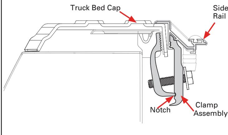
**11** Before placing the cover (A) onto the vehicle, slide two cover retainer clamps (G) into the track on the underside of the cover (A) near the cab. Confirm the cover retainer clamps fit properly into the cover rail for optimum fit. Repeat on the opposite side of the cover.
