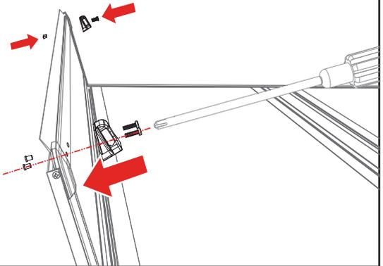
**13** Set the cover (A) in the folded position on the side rails (B & C) towards the cab of the truck. Confirm the cover is evenly spaced between the rails.
