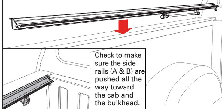
Check to make sure the side rails (A & B) are pushed all the way toward the cab and the bulkhead.
