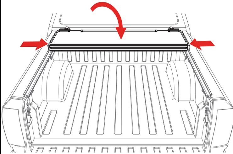
**14** Confirm the retainer clamps (G) are positioned around the side rails (B & C) correctly as shown below. Tighten the retainer clamps by turning them clockwise until the lock washer is secure.
