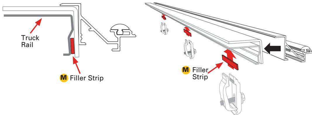
**IMPORTANT:** In order for the cover (A) to operate properly the side rails (B & C) **MUST** be square (90° angle) to the truck bed rails. This allows the rear latch to engage properly.
