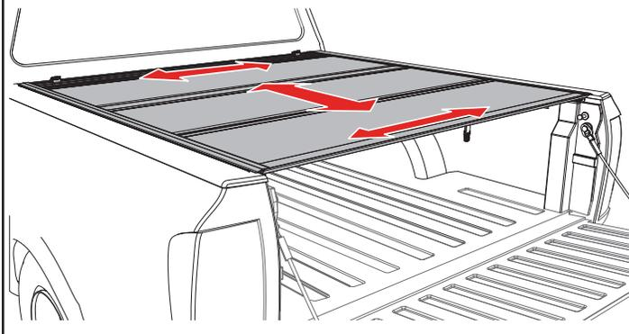
**Power Tailgates:** If your truck has a powered opening or closing tailgate ensure the tailgate functions properly with the cover closed and if needed adjust the cover towards the truck cab.
