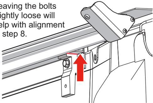
When tightening the bolts, make sure the Z-braces remain in place.
