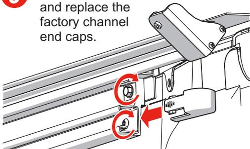
When tightening the bolts for the brackets, make sure the tonneau rail is tight up to the front of the bed.
