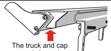
The truck and cap are not shown to demonstrate the location of the Z-braces.
