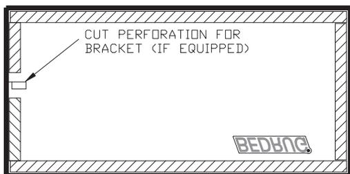
**NOTE:** Cut opening at perforation if tailgate has metal arm.
