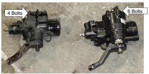
To identify this steering box, look at the top of the steering box, the old compatible unit will have four bolts fastening the top cover in place. While the newer steering box will have six. Also the sector shaft on the old compatible unit will be 7/8 thread, while the newer unit will be M30.
