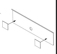
Apply single sided adhesive pads to this side of spacer. Apply BACKRACK decal
