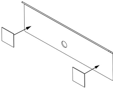
Remove 2nd side in step 4 to adhere to truck rail.
