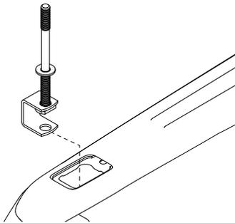
Remove rear stake pocket cover, install rear stake pocket bolt by hooking under bracket inside pocket. Hand tighten the stud thru the hole until the washer (welded to the stud) bottoms out.
