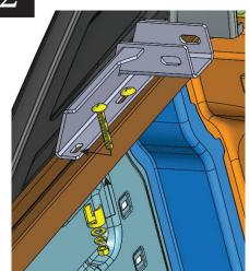
Install the carriage bolts as shown in the diagram. Finger tighten the nut with the nut spacer and washers.
