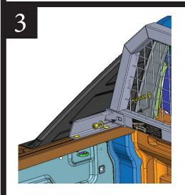
Fasten Backrack Assembly to the Rail Mount Brackets as shown.
