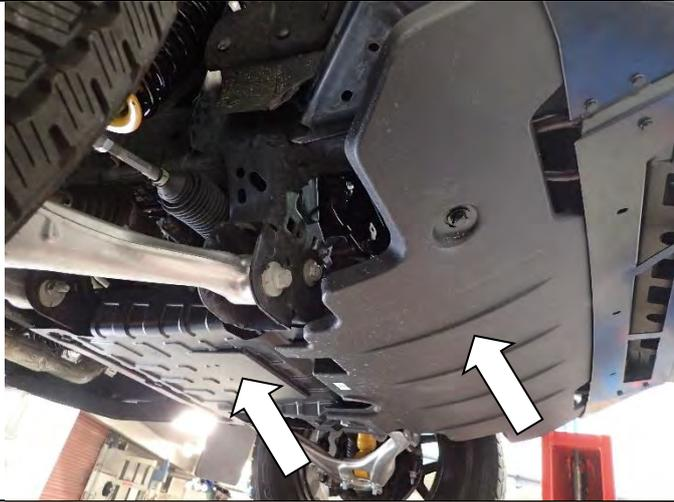
1. If fitted, remove the skids and under panels. Leave gas tank skid in place.
