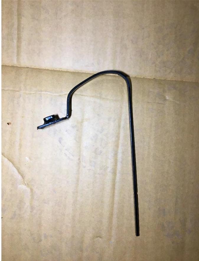
2. Start by prepping the chassis for the UVP installation. Bend 2 x M12 nut wand in the configuration shown.
