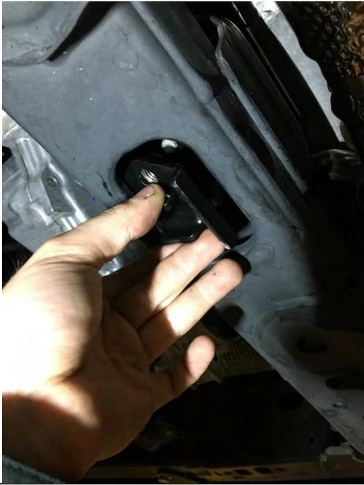
7. Insert the Internal chassis nut plate into the chassis as shown.
