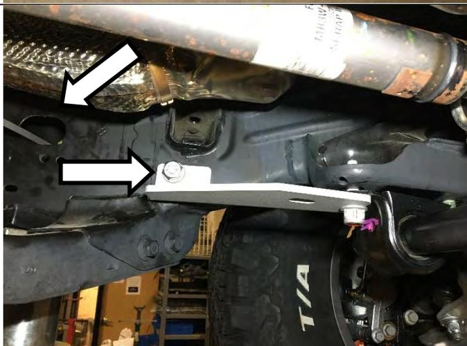
4. Insert nut wands into frame rail through large oval and around inner frame reinforcements.
