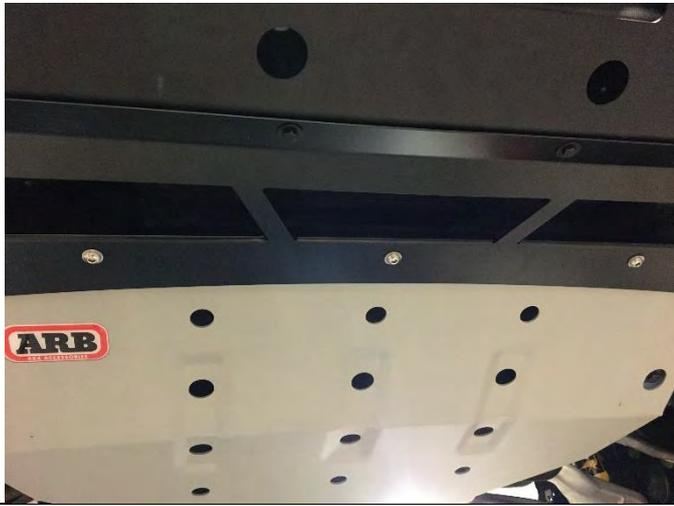
12. If fitted, install 3x M8 x 20 button heads and washers into bumper splash pan.
