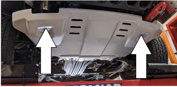
1. Remove factory front & diff stone guards from vehicle and set aside front 2 fasteners.
