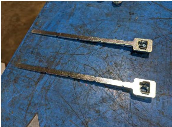
4. Position M10 cage nuts into nut plates as shown.
