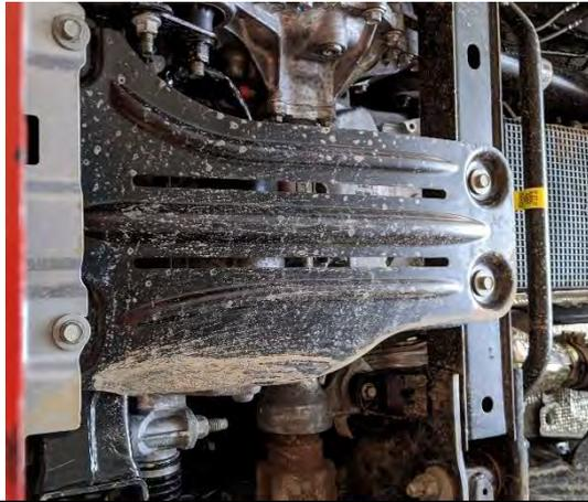
2. Remove factory transmission guard from vehicle.
