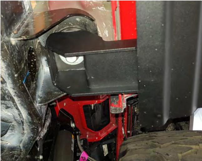
11. Fit the front mount bolt with 2 packers to secure the step while supporting the rear.
