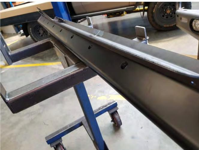
9. The edge of the step section is not straight and should have a curve when secured. (L/H side Shown)
