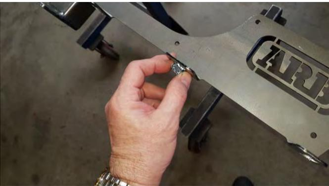
5. Clip M8 cage nuts into all slots on the R/H mount plate. Ensure they can slide freely.
