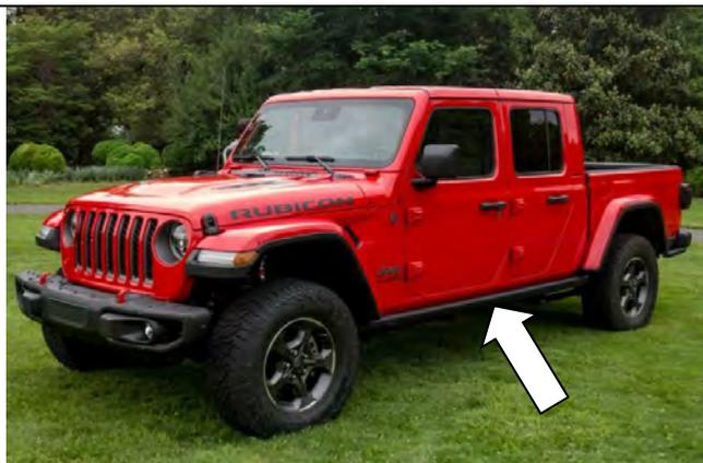
1. If fitted, remove the factory side steps retaining all fasteners.
