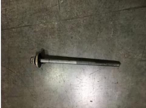
3. The rear mount is shown here, **heat and an impact wrench are needed** to remove this bolt. Take care to not melt the bushing, you will need to heat it off and on until it comes loose since it is extra-long. (bolt removed)
