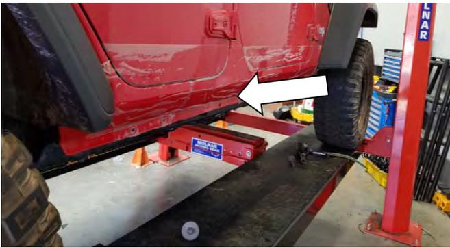
4. Protect the paint work on doors and sills both sides of vehicle. Use low tack film or similar material. (Four-door JL shown)
