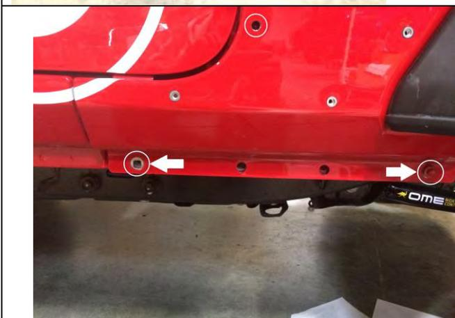
20. In order to install nutsert in the hole directly under the door hinge, the fender must first be loosened. Loosen four bolts shown in pictures before inserting nutsert.
