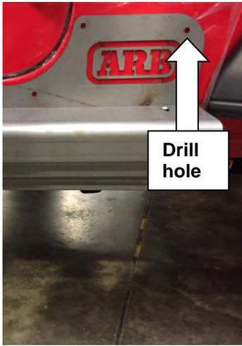
14. Drill the front hole then remove the step.
