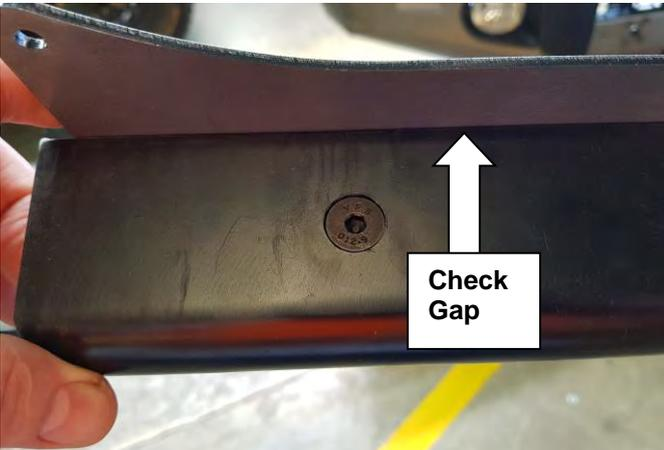
8. When tightening the countersunk screws, hold the mounting plate up against the edge of step to achieve minimum gap and tighten.
