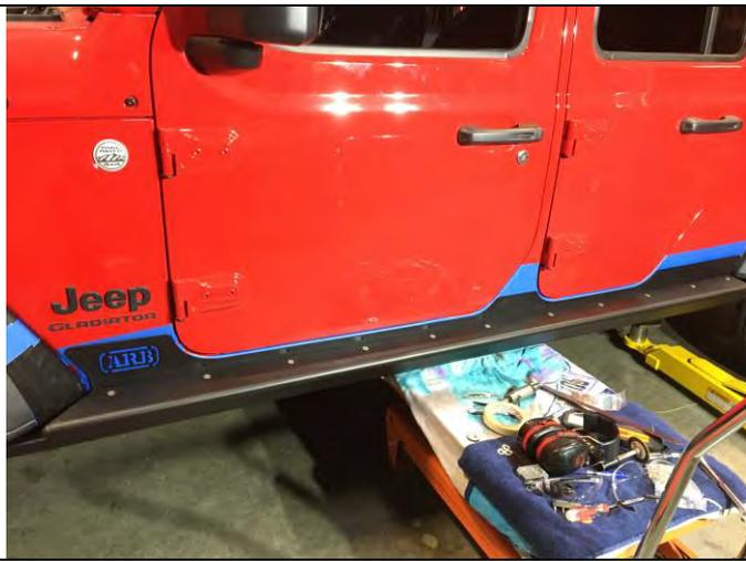
10. With either a lift table or 2 helpers, lift the assembly to the side of the car as shown. Look to make the gap along the doors even.
