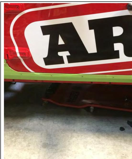
19. Use a 6mm transfer punch to mark the remaining holes, then drill using a  $\text{\O}6\text{mm}$  bit.
