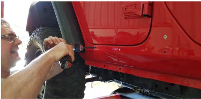
15. Drill out two pilot holes to Ø10mm to suit the M6 nutserts. (Four door shown)
