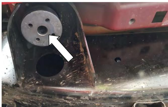
2. Remove the body mounting bolts in the front and back along the chassis.
