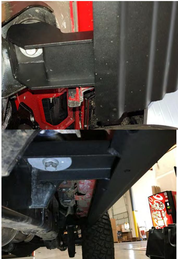
23. Refit the mount plate to the side of vehicle with M6 x 25 button head screws.
