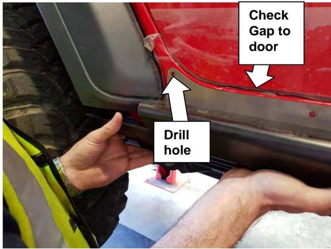
14. With the step secured against the car and the gap even use an Ø6mm drill, carefully drill hole to minimum depth at the rear of the panel as pilot for the nutsert drilling position.
