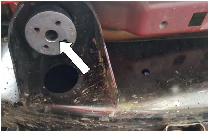
2. Remove the body mounting bolts in 3 places along the chassis. Front mount shown is the reference mount and will need no packers.
