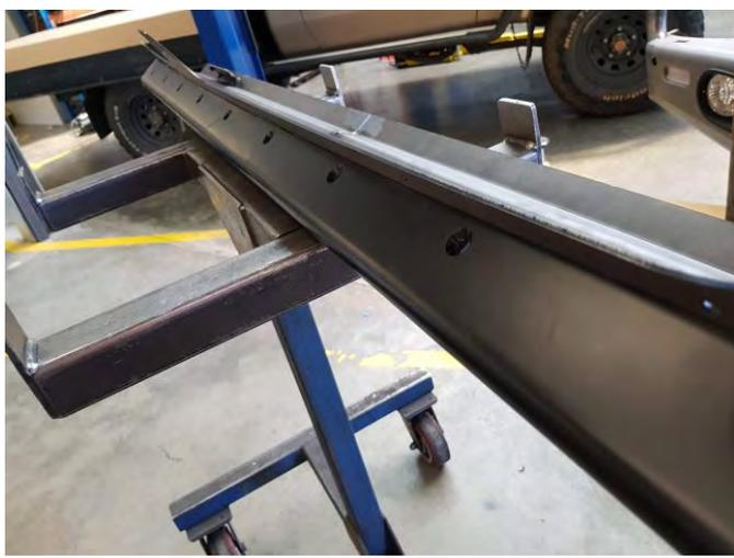
9. The edge of the step section is not straight and should have a curve when secured. (L/H side Shown)
