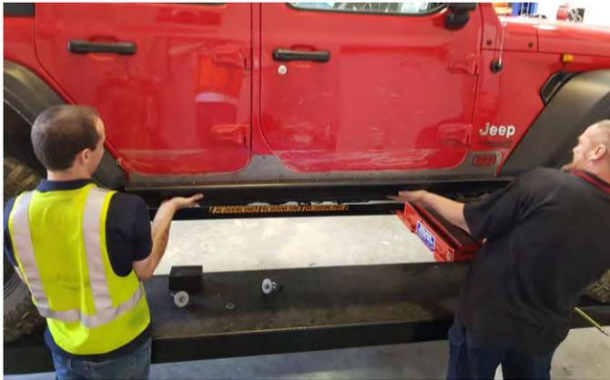
10. With 2 helpers offer the assembly to the side of the car as shown. Look to make the gap along the doors even.
