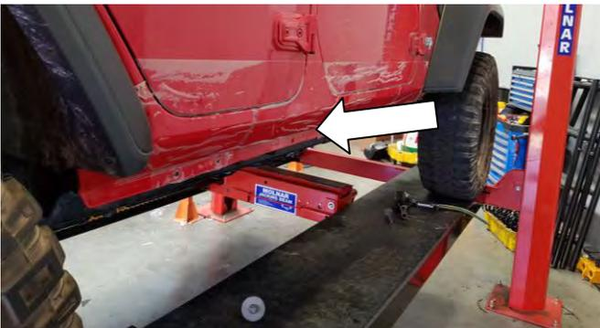
4. Protect the paint work on doors and sills both sides of vehicle. Use low tack film or similar material.
