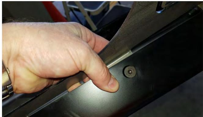
7. Fit the mount plate to the step. Start all the M8 countersunk screws
