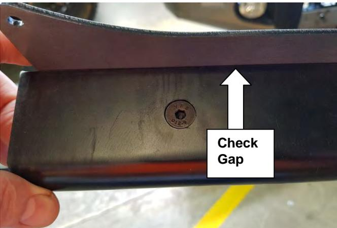
8. When tightening the counter sink screws, hold the mounting plate up against the edge of step to achieve minimum gap and tighten.
