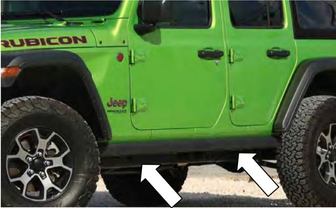
1. If fitted, remove the factory side steps retaining all fasteners.
