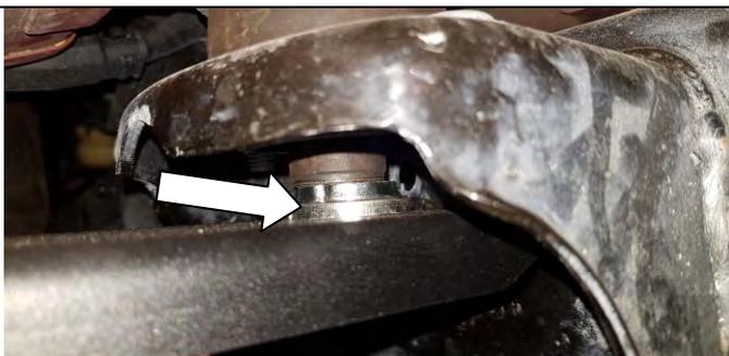
12. Insert the rear mount bolt with 2 packer washers between the mount plate and the body mount to start setup. Add or subtract spacers to level gap along bottom of the door openings.
