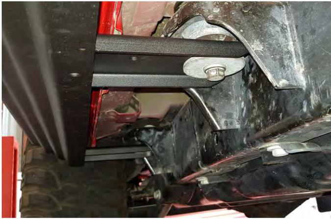
21. Run a bead of silicon sealant around the body mount plate inside surface as a seal against weather.
