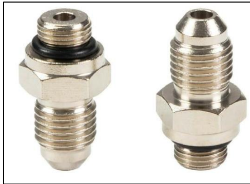
Figure 1. No sealant is required on JIC fittings or parallel threads
