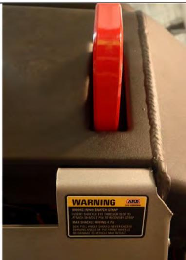
29. Fit recovery point decals to under panel directly below recovery points as shown.
