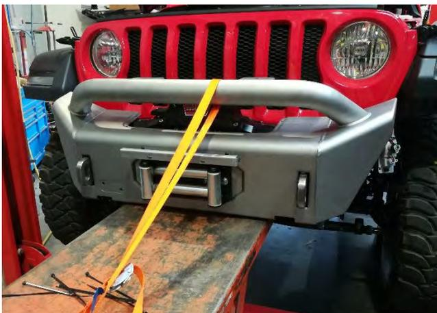
24. With the assistance of a second person and/or height adjustable trolley, carefully position the bar in front of the chassis mounts, taking care to route any winch or other accessory cables around obstacles and clear of the chassis mounting faces.
