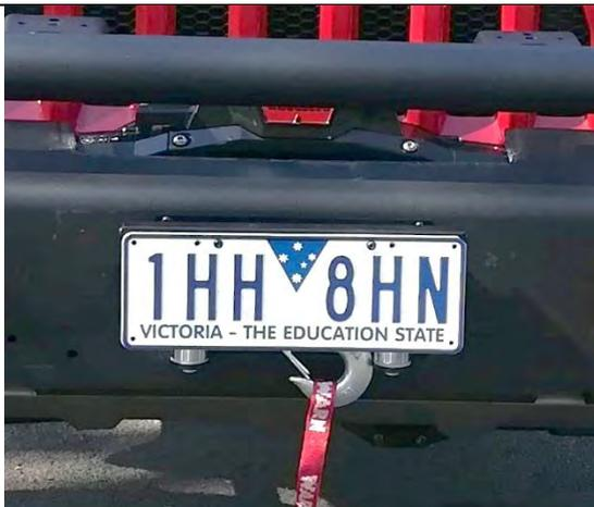
28. Fit number plate to number plate bracket using 2x M6x16mm hardware provided (if applicable).
