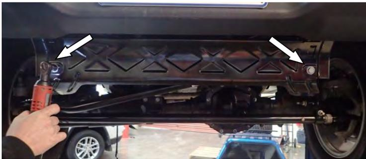
3. Remove 2x M10 SEMS from the steel front panel and discard.
