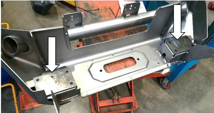
22. Secure recovery points to bar using 2x M6x20mm button head bolts provided.
