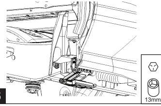
Center step pad on lower mount and scure using provided PT Screws. Tighten to 5ft-lbs using a T25 Torx bit. Verify Step pad alignment to body line of vehicle. Once step pad is in line to vehicle torque all bracket hardware to 16ft-lbs.
