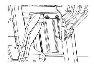
Slide assembly into position and snug bolts so frame mount of assembly is snug to bed channel. Adjust linkage assembly so its parallel to bed panel. Slide steel bracket up to frame and mark hole location to be drilled. Remove linkage assembly and pre drill using an 1/8" drill bit. Then drill to 17/32". Install rivet nut with provided steps included in rivet nut package.
