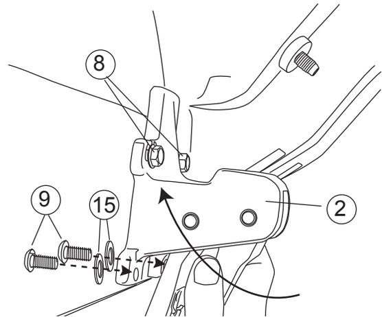
**3** Note: Excursion requires hole to be drilled in body for rear linkage. Use 25/64" Drill Bit.
