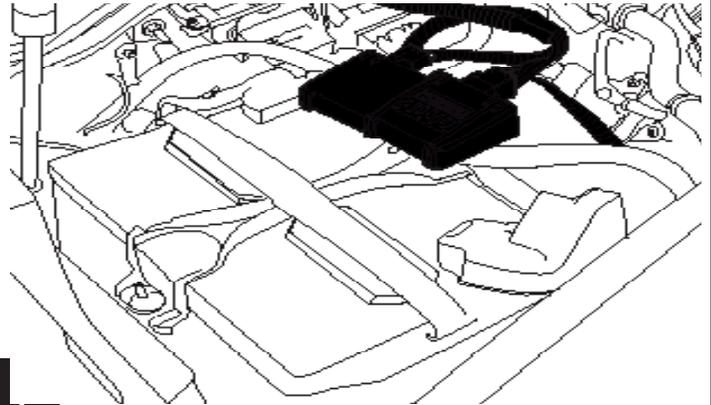
Connect power and ground for controller to battery, Red to positive and Black to the negative lead. Route harness legs down over wheel wells toward motor linkages, long leg across front and over to driver side. Secure all loose sections of the harness with cable ties.
