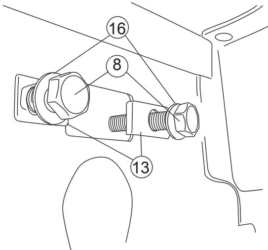
Torque fasteners to 16 ft-lbs. (22 N m).
