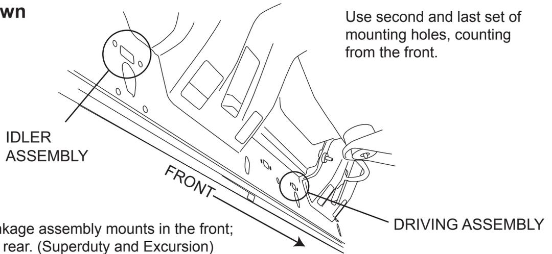
**NOTE:** Driving Linkage assembly mounts in the front; idler mounts in the rear. (Superduty and Excursion)
