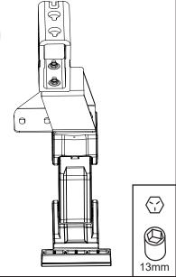
Remove factory bolt on forward most bed channel. Using supplied drill template (#14) and bolt (#10) attach template to bed channel. Make sure template edge is parallel to bed channel edge. Center punch hole, remove template, Pre drill using 1/8" drill bit. Then drill to 17/32". Install rivet nut with provided steps included in rivet nut package.
