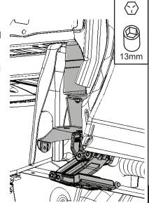
Install assembly into position. Tighten frame mount up to bed channel. Slide bracket up to frame and assemble bolt (#12) into position. Hand tighten only.
