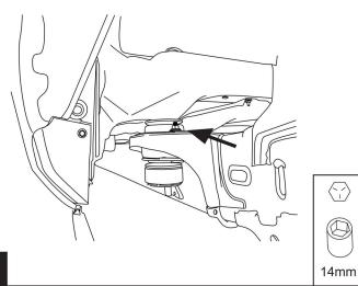
Assemble linkage to brackets as shown. Leave hardware loose to allow adjustment. Reuse nut from step 1 and attach bracket (6) to body mount as shown.
