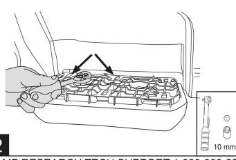
Insert reinforcement nut plate into position onto beside step sub-frame. The final position will be on top of lower shelf of the sub-frame and between the side supports.
