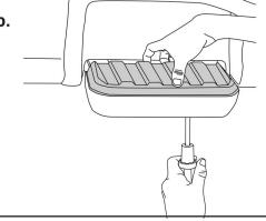
Remove bottom part of the step pad. Use ratchet to remove both bolts holding it in place.
