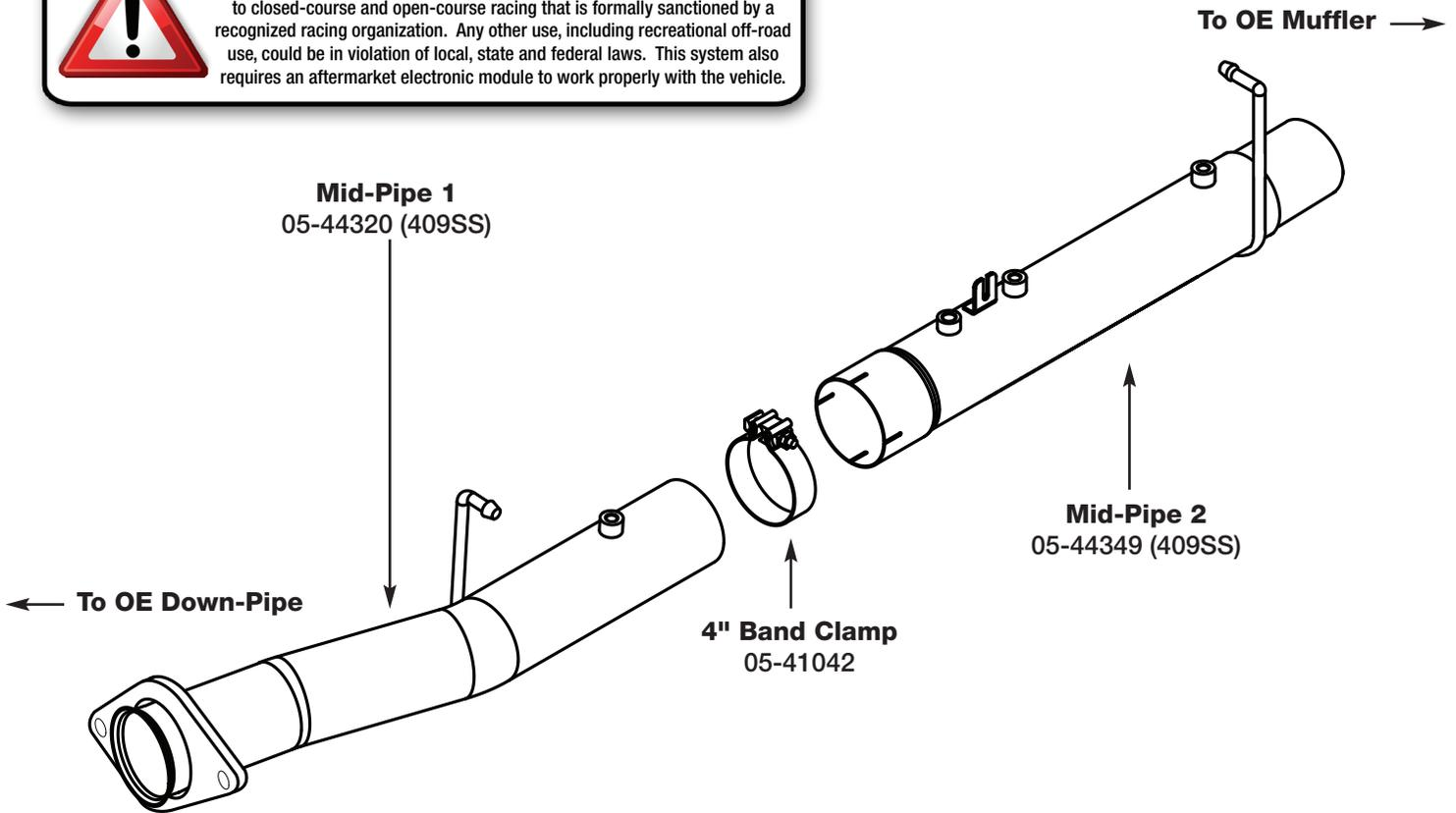
**Step 1: (Read Instructions prior to installation)** Disconnect sensors at the connections. Take caution as not to damage any sensors. Remove the CAT/DPF section of your trucks exhaust working your way forward. Take caution not to damage the factory isolation mounts as they will be reused. **It is recommended to not fully tighten the clamps until the entire system has been installed.**
