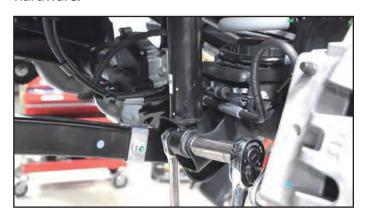
**9.** Use a 15mm wrench to remove the brake line bracket from the lower control arm. Retain the OE hardware for re-use.
