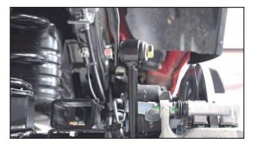
**11.Use 18mm wrenches to tighten the upper sway** link bolt. Torque to 75ft/lbs.
