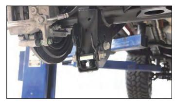
16. Install the supplied 1/2" x 1.25" bolt, washer and 1/2" nylock nut in the bottom shock mounting hole. The washer will go under the nut. Do Not Tighten.
