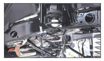
**18. Install the bump stop spacer into the lower coil** mount, using the supplied 3/8" x 3" bolt, washers, and nut through the spacer and coil mount. Tighten using 9/16" wrenches.
