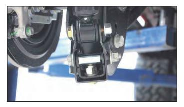
**18. Tighten the factory shock bolt using an 18mm** socket and wrench. Torque to 55ft/lbs.
