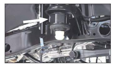
17. Re-install the coil spring.
