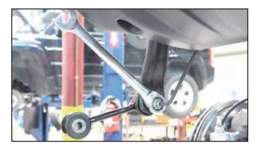
**28.** Install the new supplied bent sway link using the supplied 12mm x 65mm bolt, 1/2" washers, and lock nut. Torque to 55ft/lbs.
