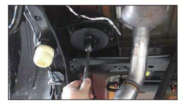
14. Install the coil spring isolator and coil spring.
