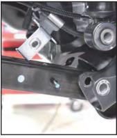
**10.** Use pliers to remove the wiring harness from the upper control arm, and to pull the axle vent tube from the differential housing.
