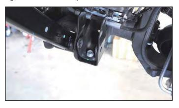
**21. Place the supplied crush sleeve into the factory** shock bracket. Install the factory shock hardware into the brackets and through the sleeve.
