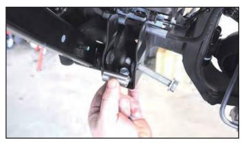
**22. Tighten the lower bolt using a 9/16" socket and** wrench. Torque to 30ft/lbs.
