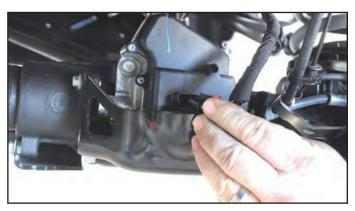
**14. Carefully lower the floor jack so that the coil** springs are at rest, neither in compression or extension. Remove the coil springs and spring isolators from both sides of the Jeep.
