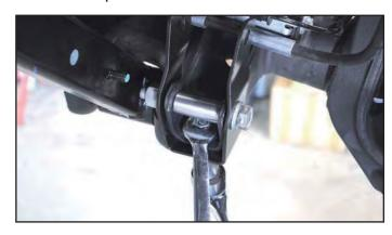
23. Use the floor jack to lift the axle housing and compress the suspension, then install the lower end of the shock into the extension bracket using the supplied 12mm x 65mm bolt, 1/2" washers, and 12mm nut.
