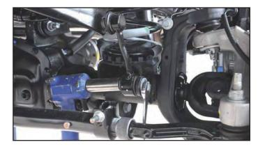
**8.** Use the 18mm socket and ratchet to remove the lower shock bolt. It may be necessary to raise the axle slightly, with the floor jack, and pull down on the shock to remove the bolt. Retain the stock hardware.
