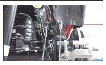
**12. Install the supplied coil spring spacer washer on** top of the coil spring pocket.
