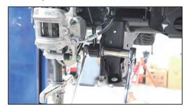
**6.** Lower the axle and remove the coil spring and coil spring isolator.
