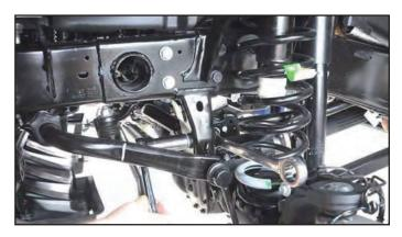
**7.** Use an 18mm socket and ratchet to remove the bottom sway bar link bolts. Retain the hardware for re-use.
