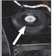
**13. Install the supplied rear coil spacer, using the** supplied 1/2" x 2.5" bolt. Tighten using a 3/4" socket. Torque to 65ft/lbs.
