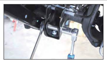
**25. Tighten the lower shock bolt using an 18mm** socket and wrench. Torque to 55ft/lbs.
