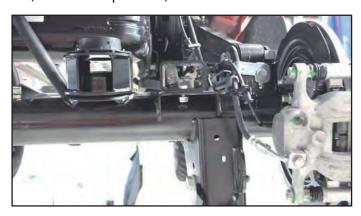
**8.** Use a 9/16" wrench and socket to torque the hardware to 30ft/lbs.
