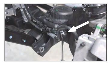
**16.** Install the supplied spring spacer with coil spring isolator under the spacer.
