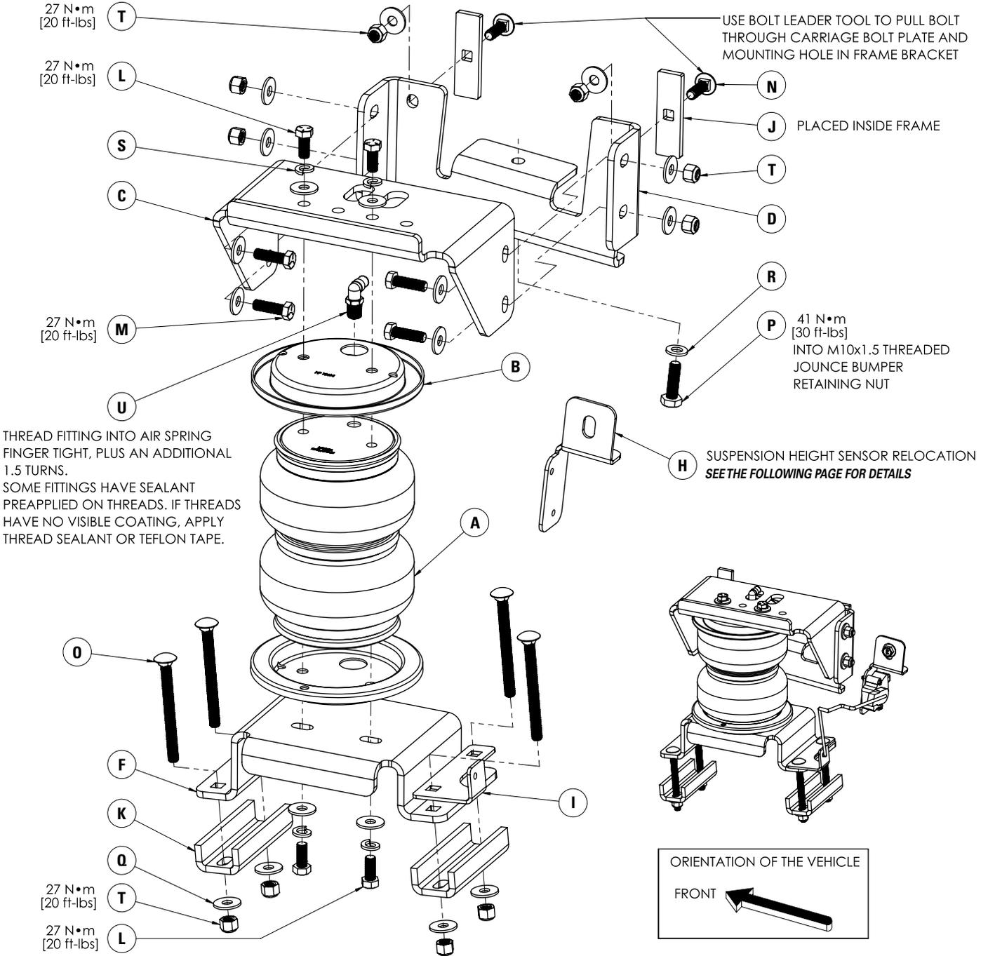
**RIDE HEIGHT SENSOR ASSEMBLY SHOWN: (FOR VEHICLES WITH RIDE HEIGHT SENSOR ONLY)**
