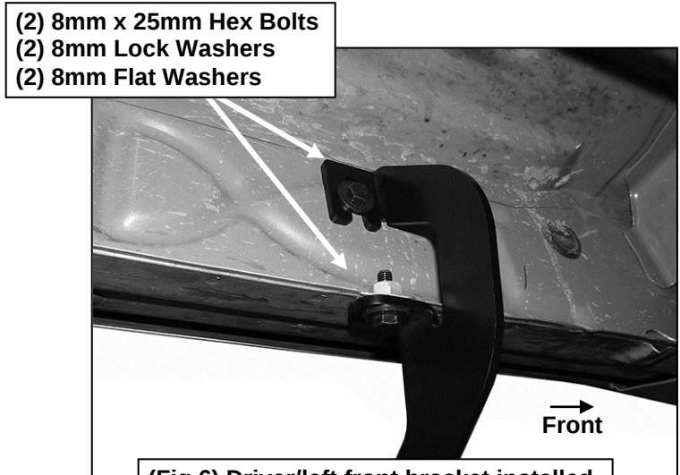
(Fig 6) Driver/left front bracket installed
