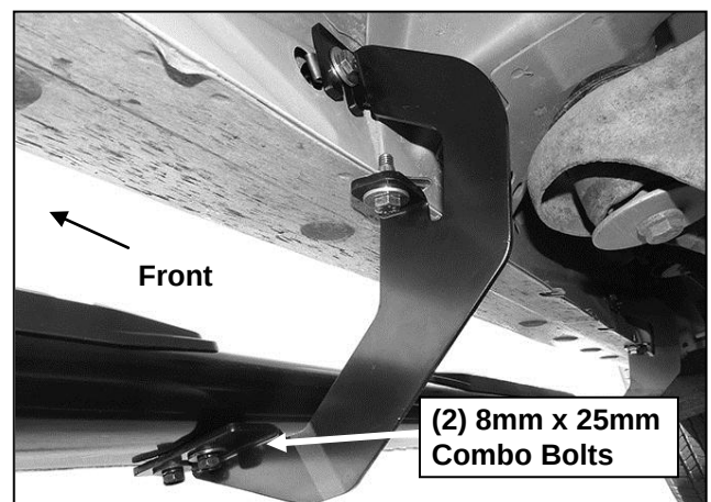
(Fig 20) Passenger/right center bracket installed
